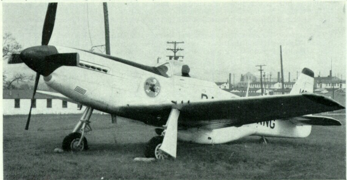
ETF-51D-25NT of Air National Guard. Tall fin was introduced on the P-51H and several F-51Ds were retro-fitted during the early post-war period. Note "Bald Eagle" motif ahead of cockpit.
