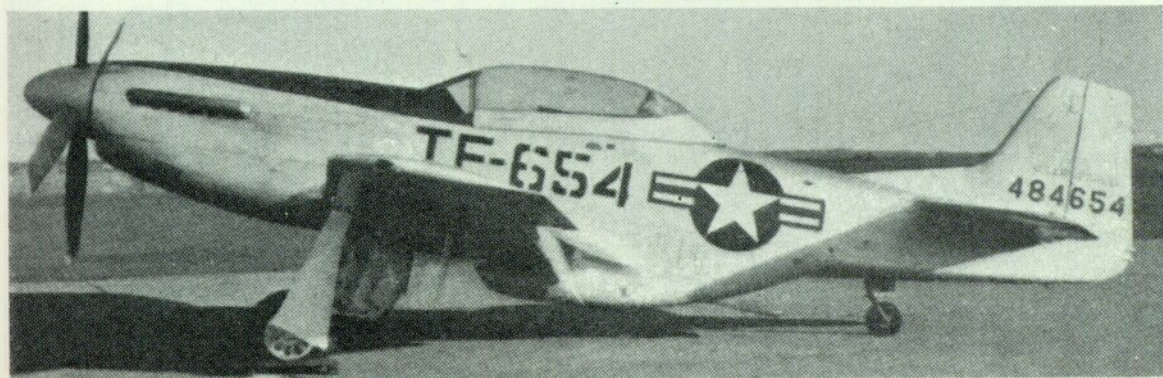
TP-51D trainer with dual seats under single bubble canopy.
