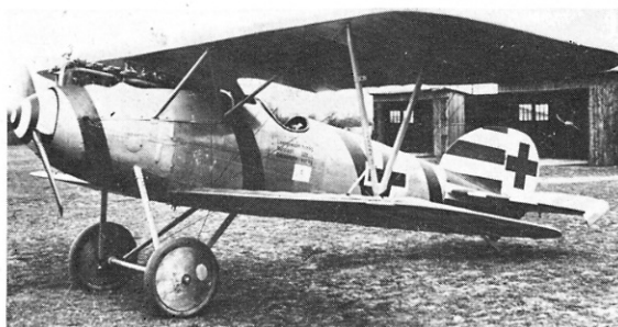
This Albatros D Va—D6553/17, (O.A.W.), thought to be Jasta 4, was a Schneidemühl-built machine. Note auxiliary strut from interplane strut to leading-edge. (Photo: Egon Krueger)
