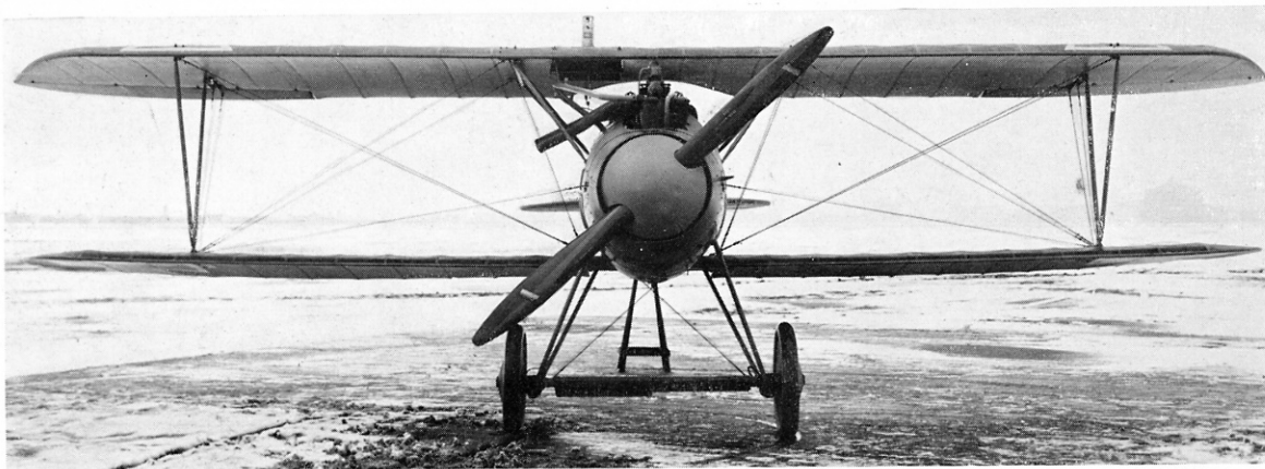
Sleek lines of the D Va are displayed in this head-on view. Note absence of auxiliary strut.
