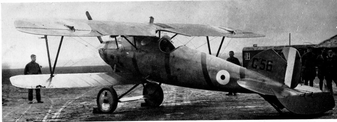
Captured Albatros D V, D2129/17, with spiral ribbon marking. Note British A.S.I. pitot head on port interplane struts.
