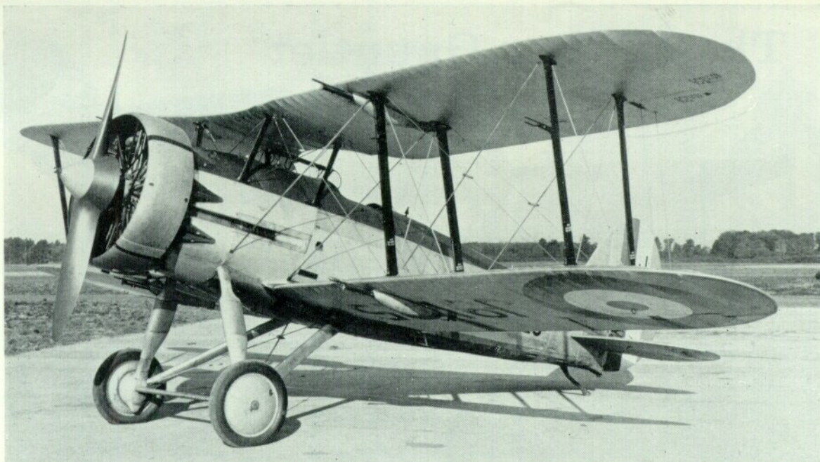
The Gloster S.S.19, J9125, fitted with the six-gun armament of four Lewis guns on wings and two Vickers guns in fuselage. (Air Ministry photo)
