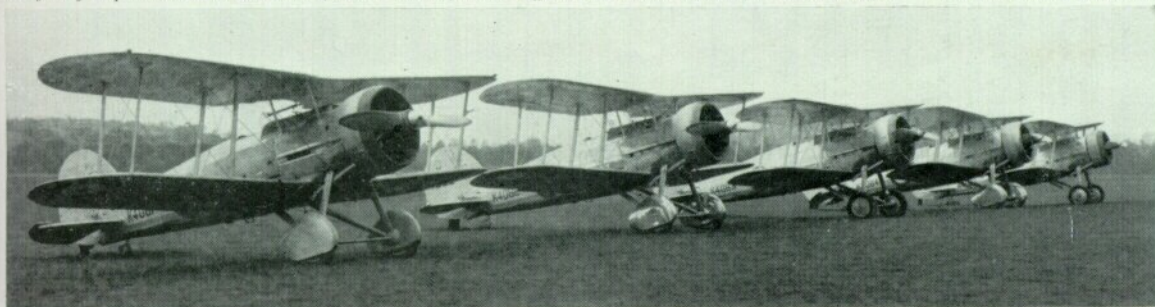
The first five production Gauntlet Is (K4081-K4085). Note differences in undercarriage wheel fairings. (Gloster Aircraft photo)
