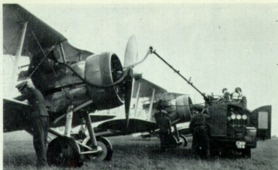
Gauntlet IIs being refuelled in pairs. ("Flight" photo)
