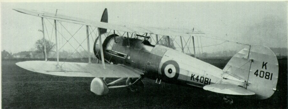
Two further views of the first production Gauntlet I. Note Vickers gun troughs in fuselage and sight ahead of windscreen. (Air Ministry photos)
