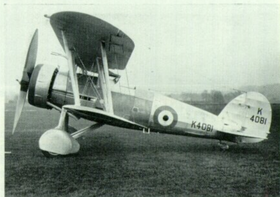
Two further views of the first production Gauntlet I. Note Vickers gun troughs in fuselage and sight ahead of windscreen. (Air Ministry photos)
