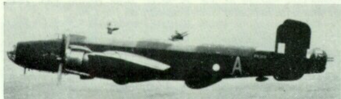
B.VI PN369, operating in S.E.A.C., seen on a mission against the Japanese. Note streamlined fairing beneath rear fuselage. (Photo: Imp. War. Mus.)
