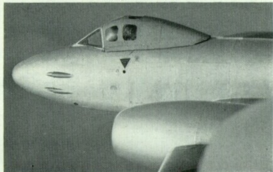
High-altitude tests were carried out with VZ439, fitted with strengthened hood.
