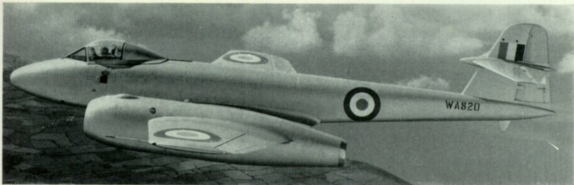
The most powerful Meteor 8 flown was WA820, fitted with two Armstrong-Siddeley Sapphire engines providing 15,200 lb. s.t. (Photo: Hawker Aircraft)
