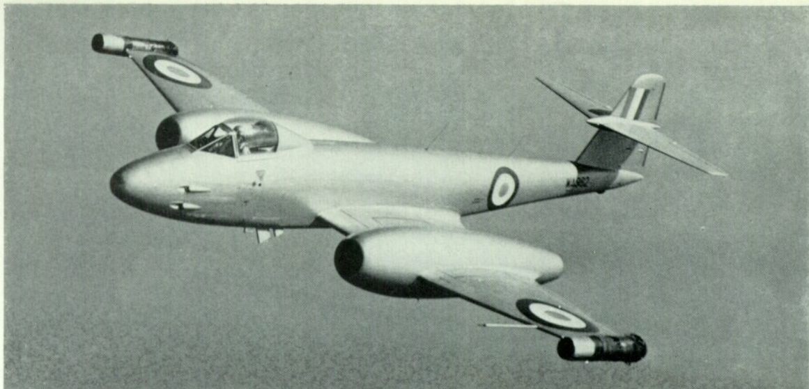
WA982 was used to flight test the Rolls-Royce Soar engine, weighing a mere 275 lb. Only one Soar was installed, the port fixture being a dummy. (Photo: Rolls-Royce)
