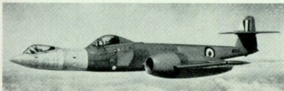
Interesting F.8 conversion was WK935. Second cockpit accommodated pilot in prone position.
