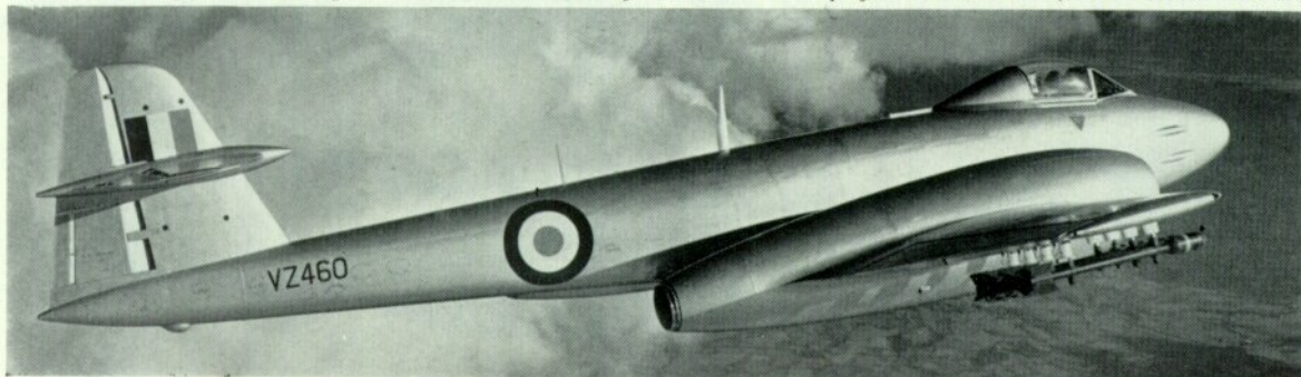
Meteor VZ460 of the Central Fighter Establishment was used for tests with rocket projectiles and bombs. (Photo: Gloster Aircraft)
