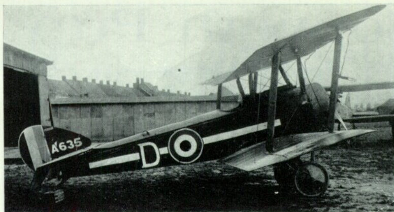
A635 of No. 66 Squadron was also captured intact by the Germans and is here seen with the elevator control cables and air-speed indicator leads disconnected. The squadron marking has been somewhat roughly applied, and the proportions of the fuselage rounder are interesting. (Photo: Egon Krueger)
