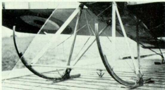
This Pup had rigid skids with flexible forward extensions, three V-shaped horns for fore-and-aft arrester cables, and a hook for athwartships cables.
