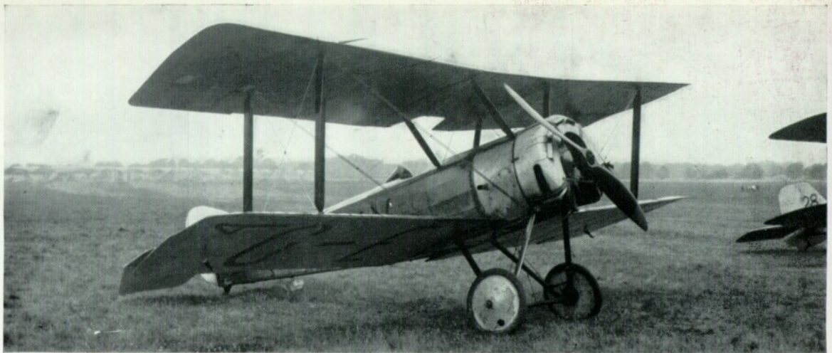
Although G-EAVX (ex B1807) had an 80-h.p. Le Rhône engine it was fitted with the Monosoupape-type cowling; it also had a head-rest behind the cockpit. This photograph was taken at Hendon; the occasion was the 1921 Aerial Derby, 16th July 1921. (Photo: "Flight" International)
