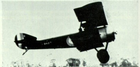
Below: One of the prototype Pups, 9497 (marked N9497) was used in early deck-landing experiments and is here seen with its arrester hook lowered, approaching the dummy deck at the Isle of Grain. The airscrew guard can just be distinguished.
