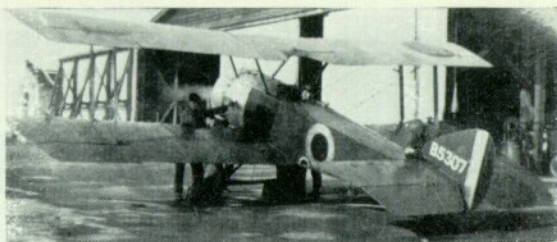
Night-flying Pup with partly obliterated national markings, fitted with navigation lights. (Photo: via C. A. Nepean Bishop)
