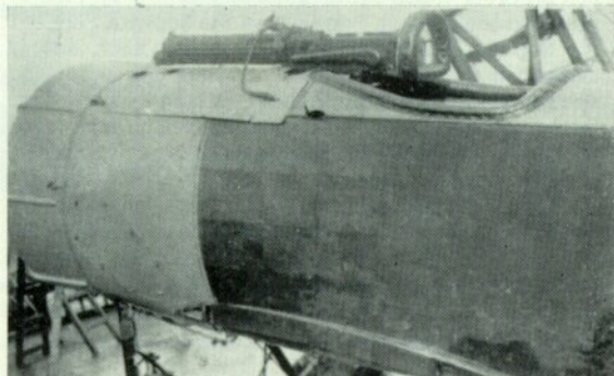
Left: The installation of the 100-h.p. Gnôme Monosoupape, here seen on a Whitehead-built Pup. Right: Fuselage detail of Whitehead-built, Monosoupape-powered Pup. The hydraulic lead and trigger motor of the Constantinesco C.C. synchronising mechanism can be seen.
