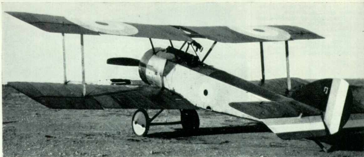
One of the Beardmore-built Pups of "C" Squadron, R.N.A.S., Imbros, armed with Vickers and Lewis guns.
