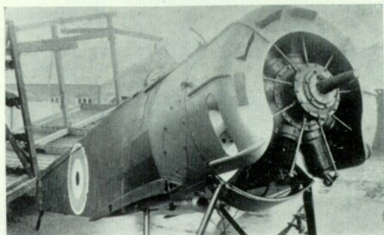
Left: The installation of the 100-h.p. Gnôme Monosoupape, here seen on a Whitehead-built Pup. Right: Fuselage detail of Whitehead-built, Monosoupape-powered Pup. The hydraulic lead and trigger motor of the Constantinesco C.C. synchronising mechanism can be seen.
