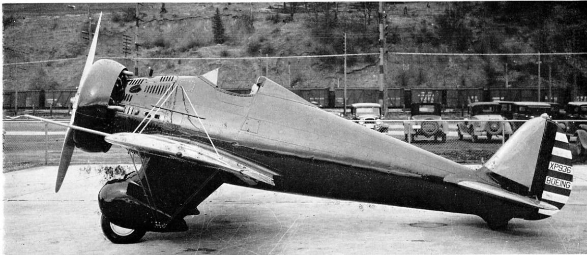
The first Boeing 248 before purchase by the Army Air Corps and carrying the designation of XP-936. Note small headrest and wheel pants projecting behind landing gear legs. (Photo: Boeing)
