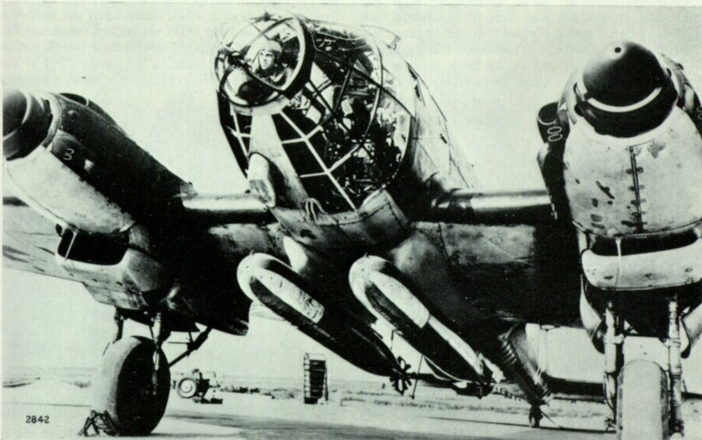
He 111H-6 of I/KG 26 "Löwen Geschwader" with practice torpedoes slung beneath the wing-roots. (Photo: Real Photographs)
