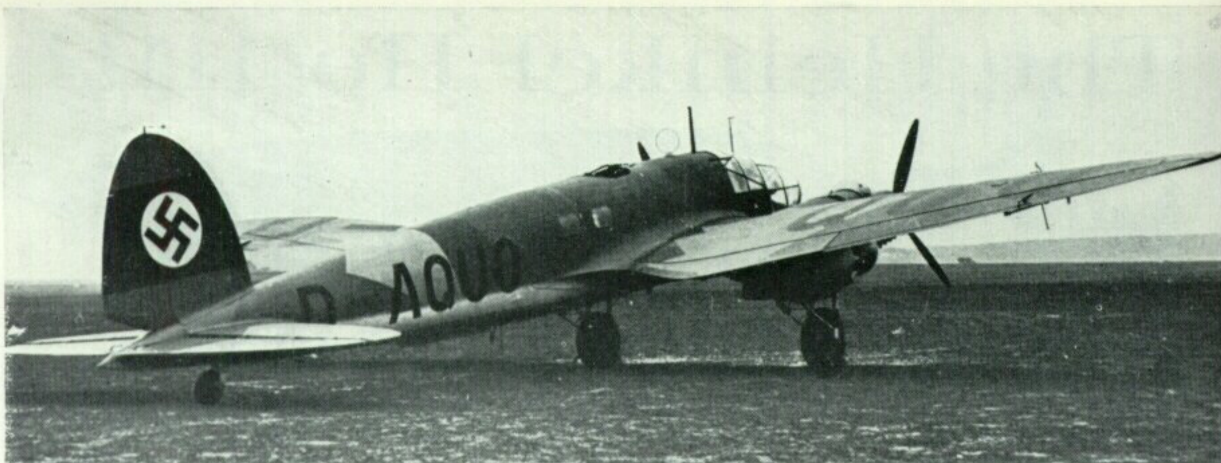
The He 111V-8, D-AQUO, which was the test-bed for the "glass-house" nose section.
