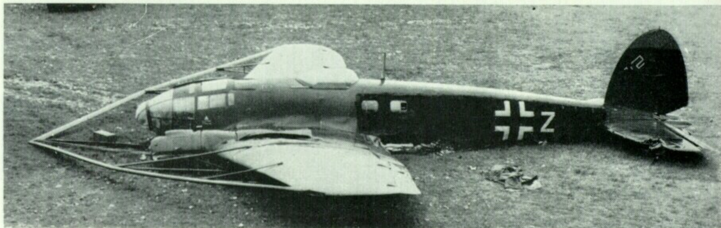
The He 111H-8 was simply an H-3 or H-5 variant with the 550 lb. balloon-cable fender/cutter installed. Note the temporary night-camouflage applied to this aircraft. (Photo: Imperial War Museum)
