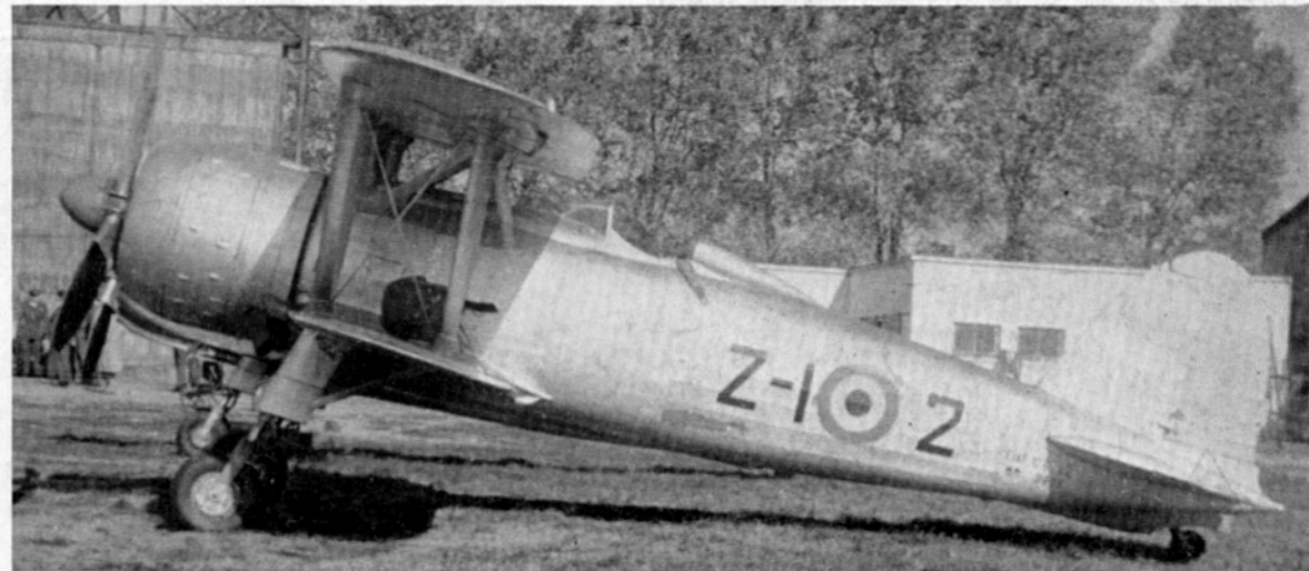
Wheel spats have been removed from this C.R.42, pictured near Milan in the early post-war years.
