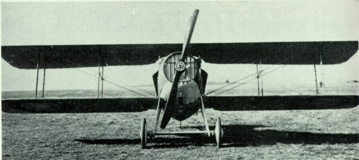
Head-on view showing the narrow-chord propeller. Below: Three-quarter rear view shows the aileron bell crank on the bottom of the outer rear strut. (Photos: Musée de L'Air)
