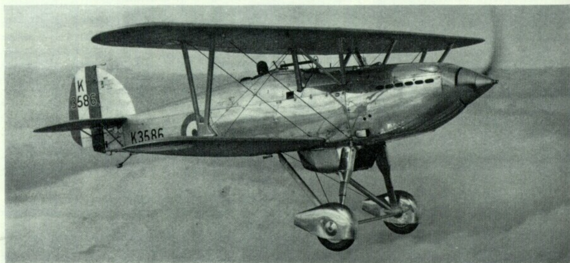
The High Speed Fury with Kestrel VI S engine, tapered wing and Vee interplane struts.
