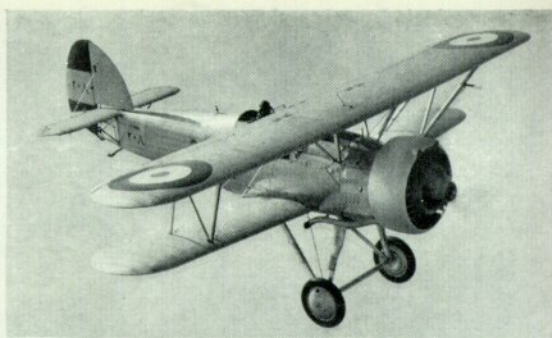
The Persian Fury re-engined with a Bristol Mercury engine. ("Flight" photo)
