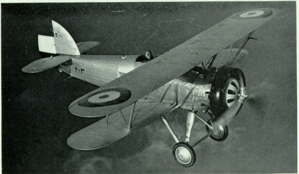
Below: Persian Fury with Pratt & Whitney Hornet engine and Hamilton 3-blade propeller. ("Aeroplane" photo.). Top of page, left: The first Persian Hornet Fury with the standard Watts wooden propeller. Right: Head-on view of the Persian Fury with Hamilton 3-blade propeller.
