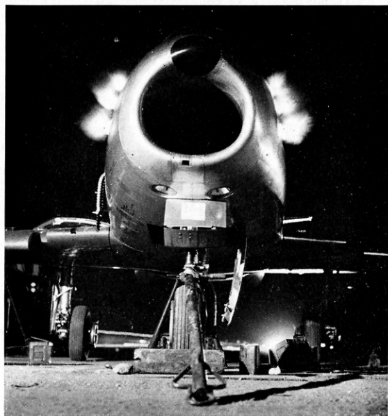
Night gun firing tests. Note landing lamps under air intake.
