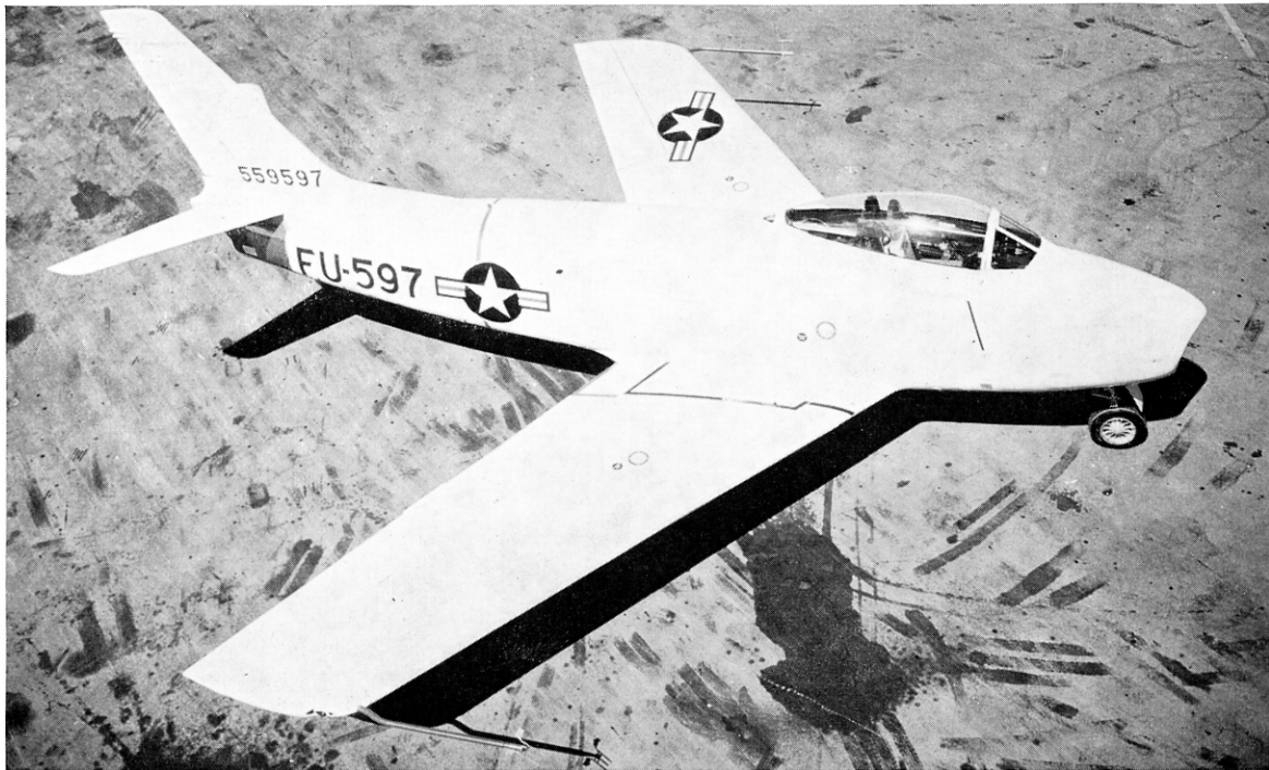
The prototype F-86A (XP-86) in the white overall finish applied for early trials.
