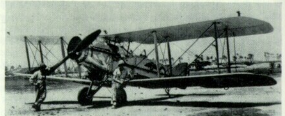
In service in India, F4349 displays some of the impedimenta with which the post-war Bristol F.2B was encumbered. This aircraft has the underslung auxiliary tropical radiator, an adjustable-pitch airscrew and navigation lights. (Photo: D. P. Woodhall)
