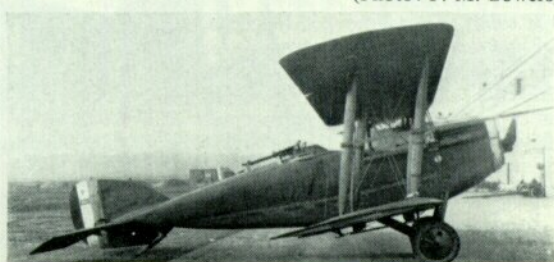
Left: The first U.S. XB-1A, S.C.40125, with the semi-monocoque fuselage developed at McCook Field. This fuselage weighed only 165 lb.; that of the U.S.A. O-1 weighed 275 lb. Right: This XB-1A, A.S.64177 (P-205) had its lower wing faired into the fuselage. (Photo: P. M. Bowers)
