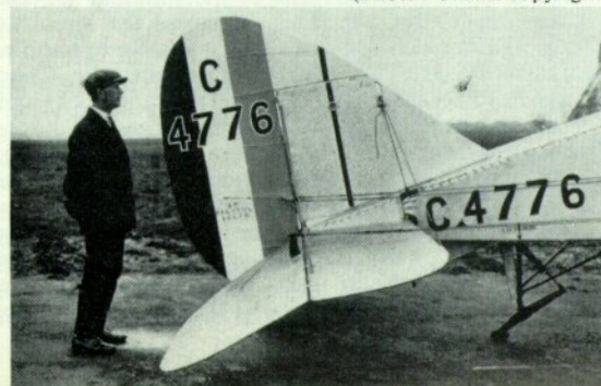
Above: Post-war use of the Bristol F.2B in India and the Middle East led to cooling problems that were investigated at Farnborough. One attempted solution was this liberally-louvered cowling, almost certainly on C4654, photographed on 29th April 1923. (Photo: Crown copyright); Below: The greatly enlarged upper fin and rudder fitted in 1920 to the Puma-powered Bristol Fighter C4655 were similar in outline to the original surfaces. At Farnborough a few years later C4776 was fitted with revised vertical surfaces incorporating a balanced rudder, foreshadowing the tail unit of the Bristol Fighter Mk. IV. This photograph is dated 23rd March 1925.
