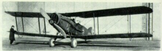
Bristol F.2B Mk. II with oleo undercarriage, enlarged tyres, flare brackets and post-war radiator shutters, 1920. This aircraft, J6790, was tested at Marletsham Heath later became G-ACCG, and survived until 1939.
