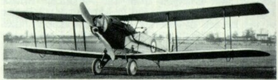
The prototype Mk. IV, H1417, had square-tipped upper wings and its upper ailerons were linked to the slats.
