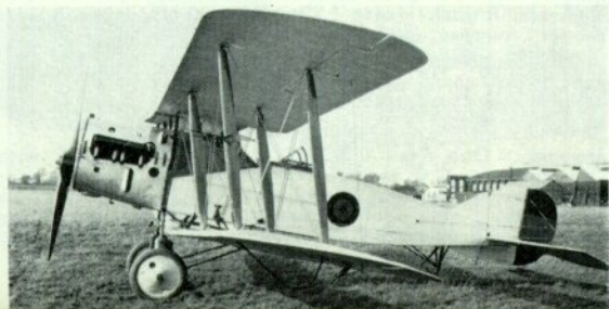
Above: Possibly a SABCA-built Bristol F.2B, this was No. 45 of l'Aéronautique Militaire Belge, with 300-h.p. Hispano-Suiza engine, oleo undercarriage and horn-balanced rudder. Below: One of twelve new-built Bristols supplied to Spain in 1924 with 300-h.p. Hispano-Suiza, oleo undercarriage and Frise ailerons.
