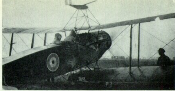
Left: A few Falcon-powered Bristol F.2Bs had radiators of increased area that substantially altered the shape of the nose. This one was photographed at the Isle of Grain shortly after the Armistice; another was at Cranwell in August 1919. Right: In the early post-war years experiments were conducted with free-flying target gliders, one of which is seen here on a Bristol F.2B. A larger type of glider was launched from a Westland Walrus.
