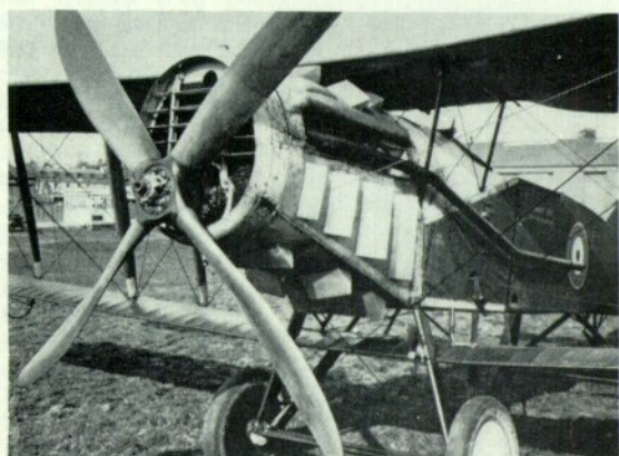
Above: Post-war use of the Bristol F.2B in India and the Middle East led to cooling problems that were investigated at Farnborough. One attempted solution was this liberally-louvered cowling, almost certainly on C4654, photographed on 29th April 1923. (Photo: Crown copyright); Below: The greatly enlarged upper fin and rudder fitted in 1920 to the Puma-powered Bristol Fighter C4655 were similar in outline to the original surfaces. At Farnborough a few years later C4776 was fitted with revised vertical surfaces incorporating a balanced rudder, foreshadowing the tail unit of the Bristol Fighter Mk. IV. This photograph is dated 23rd March 1925.
