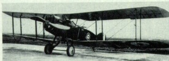
Above: The final Arab installation, using a radiator of the shape designed for the 300-h.p. Hispano-Suiza, here seen on F4640. (Photo: Imp. War Mus.)
