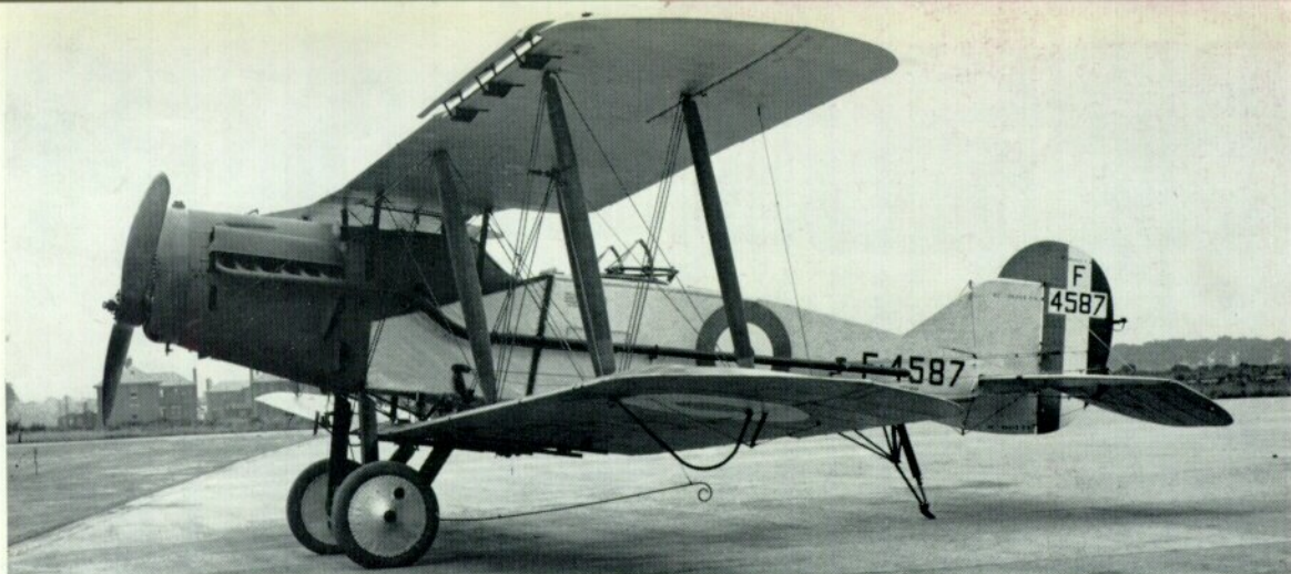
The standard Bristol F.2B Mk. IV had automatic slots on mainplanes of standard plan-form, strengthened undercarriage and fuselage, an enlarged upper fin and horn-balanced rudder.
