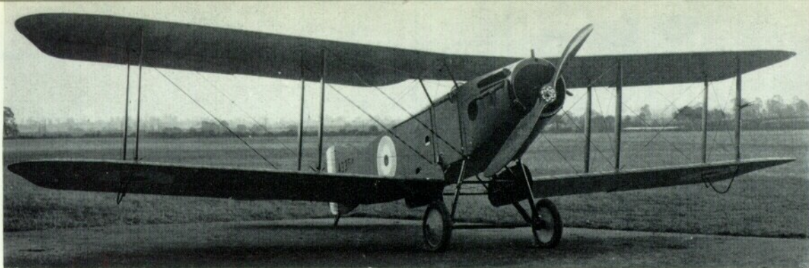
The second F.2A prototype, A3304, with 150-h.p. Hispano-Suiza, in its original form.
