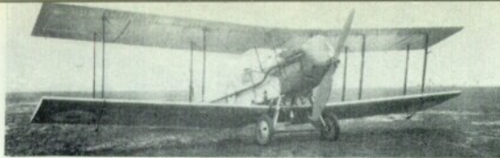
Dated 6th January 1930, this photograph depicts J6721, perhaps the most extensively modified Bristol F.2B of all. It had R.A.F. 34-section wings of steel construction embodying leading-edge condensers for the experimental evaporative cooling system fitted to the engine, which drove a Leitner-Watts adjustable-pitch airscrew. The wings had increased gap and were mounted at a large angle of incidence. (Photo: Crown copyright)
