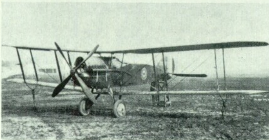
Left: One of the R.A.E.'s experimental Bristols was A7260, here seen with a 200-h.p. R.A.F. 4d engine. It was used in 1918 in tests of the Calthrop A.1 parachute, and in comparative trials with other R.A.F. 4d F.2Bs that had single-bay and three-bay wings. (Photo: P. L. Gray); Right: This U.S.A. O-1 had two radiators mounted in flank positions in line with the rear centre-section struts. At a later stage a single radiator was mounted on the centre section; it is believed an underslung radiator was tried. (Photo: P. M. Bowers)
