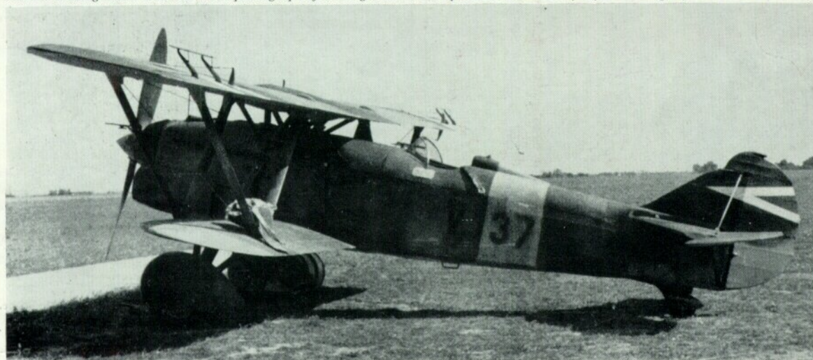
Tab and bracing detail is visible in this photograph of a Hungarian C.R.32 quarter trainer in early-style markings. (Photo: via R. Ward)
