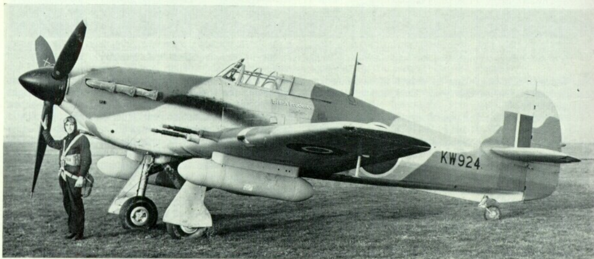
Late-series presentation Hurricane IIC "British Prudence" with two 44-gallon drop tanks. (Photos: Hawker Siddeley Aviation)
