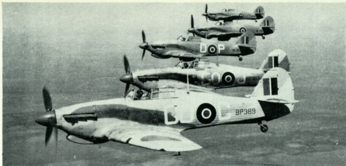
A formation of tropical Hurricane IICs. The three aircraft farthest from the camera are presentation machines commemorating the three MacRobert brothers, and outboard cannons of the nearest aircraft have been deleted in the interests of performance.
