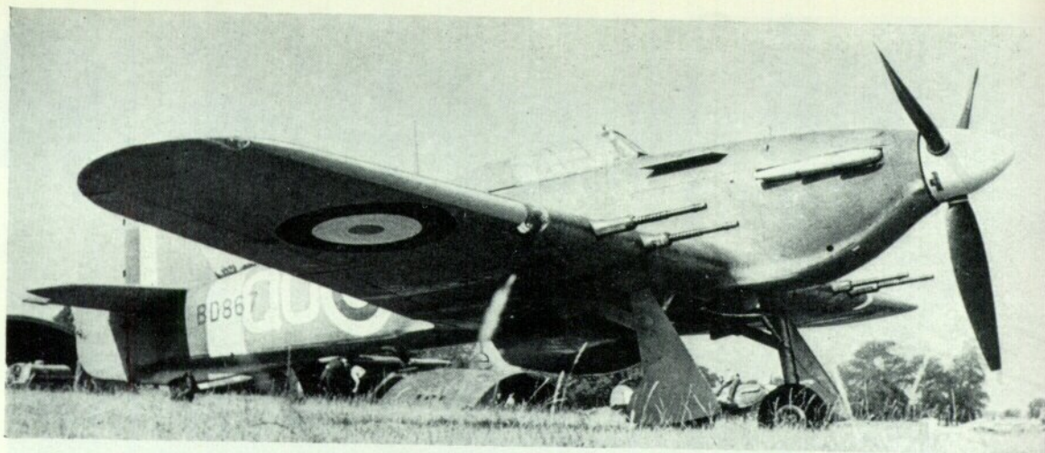
An early series Hurricane IIC of No. 3(F) Squadron in North Europe day camouflage of 1941. The exhaust shield was an "optional fit".
