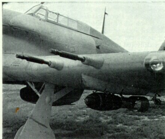
Close-up of 20 mm. gun installation of Hurricane IIC.
