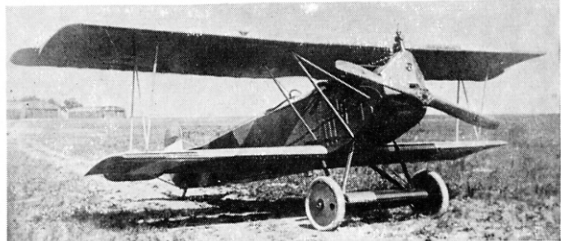
Fokker D VII built by Allgemeine Ungarische Maschinen Fabrik A.G. (M.A.G.) of Budapest. It was fitted with 210-h.p. Austro Daimler engine and radiator similar to the type used on Austrian Berg D I fighter. (Photo: Pavel Vancura)
