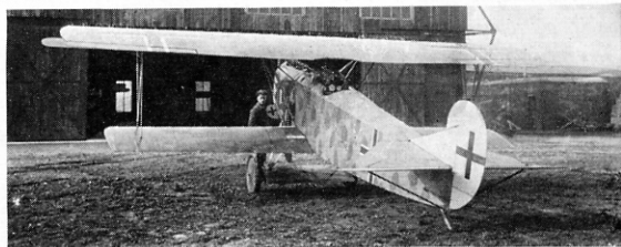
A mint product of the Ostdeutsche Albatros-Werke (O.A.W.) at Schneidemühl. Fokker D VII (O.A.W.) 6376/18. Note ex-works white fin and rudder. (Photo: Egon Krueger)
