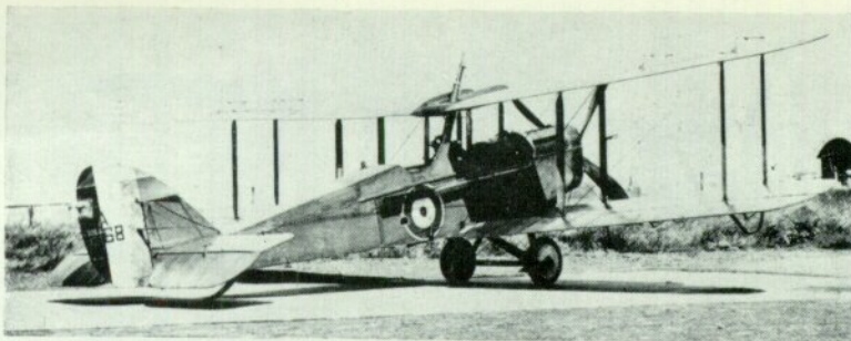
A2168 with 1½-pounder C.O.W. gun firing upwards through the centre section for anti-airship duties.
