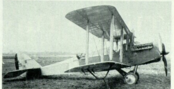
Also photographed at Orfordness. A2129 was the subject of the Martlesham trial report No. M.83. Its engine was a 250-h.p. Rolls-Royce Mk III (284-h.p. Eagle III), W.D.10071.
