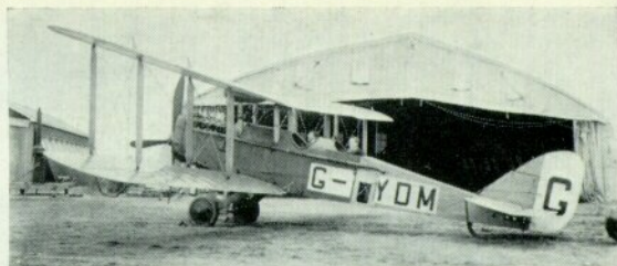
One of the so-called Canadian D.H.4Bs with the pilot's cockpit behind the wings, G-CYDM was used for photographic-survey work and is seen here with a camera port in the fuselage side. Originally F2706, this D.H.4 was taken on C.A.F. strength on 19th April 1921 and was not struck off until 30th November 1928. (Photo: via K. M. Molson)
