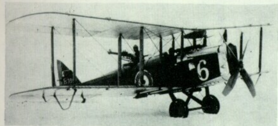
Left: B3957 was one of the N-series Westland-built D.H.4s that were transferred to the R.F.C. It retained the two Vickers guns; in this photograph it is seen with twin Lewis guns on the Scarff mounting and two T.W.R. parachute flares on the under-wing bomb ribs. Right: Subject of Martlesham report M.92, A2168 had the R.A.F.3a engine. Its Scarff ring had been raised several inches above the upper longerons. This photograph was made at Martlesham Heath in April 1917.
