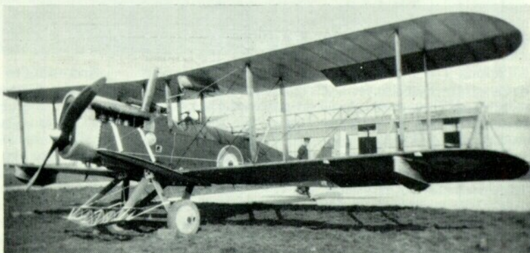
The single-surface hydrovane later fitted to the D1769. Photograph dated 16th August 1918.
