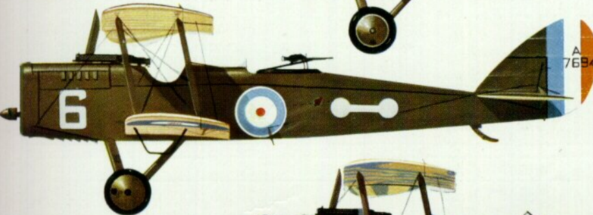
D.H.4, A7459, specially modified and camouflaged for projected photo-recce of Kiel Canal, summer 1917. Serial number overpainted.
