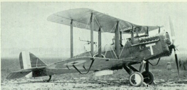
In No. 202 Squadron, 'A' Flight was known as the Photographic Flight, 'B' Flight as the W/T Flight, 'C' Flight as the Escort Flight. This Eagle VIII D.H.4 of 'A' Flight had a fairing under the fuselage housing a large camera; several other D.H.4s of this unit had similar fairings. This D.H.4 was the aircraft usually flown by Captain Warne-Brown, D.S.C., and is here seen at Bergues.
