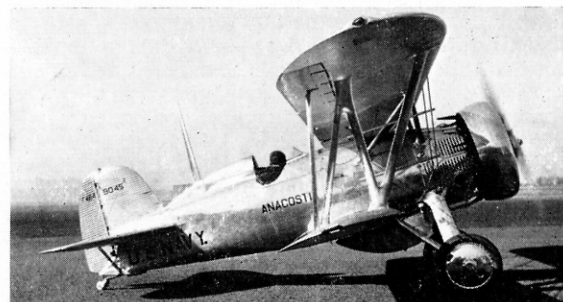
F4B-4 assigned to Naval Air Station Anacostia, with special polished Alclad finish used only at that station. (Photo: P. M. Bowers)
