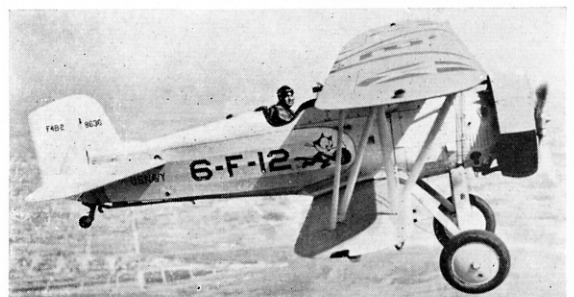
Air shots of F4B-2s show how undercarriage wheels drop in flight. Right illustration is of 8638 (VF-6B) of Fighting Squadron 6, 3rd aircraft of 4th Section.
