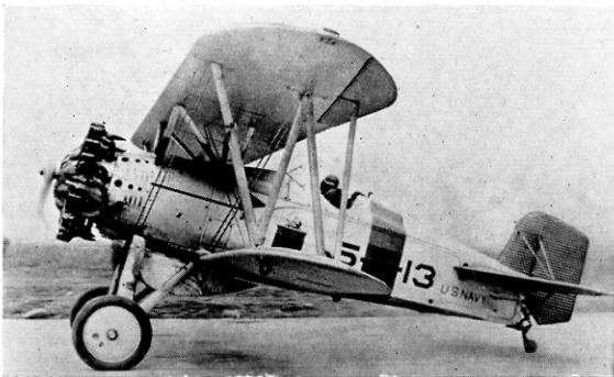
Production F4B-1, Boeing Model 99, as delivered to Navy squadron VF-5. Engine cylinder streamline fairings of original installation deleted after short period of service.
