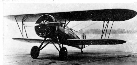
Left: Fourth production F4B-1 was converted to special unarmed executive model for Assistant Secretary of Navy for Sir Douglas Ingalls, under designation of F4B-1A. (Photo: U.S. Navy.) Right: In their declining years F4B-1s were fitted with 4B-2 ring cowlings and 4B4 vertical tail surfaces. (Photo: E. M. Sommerich)
