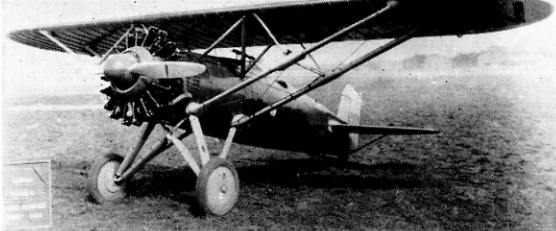
Boeing Model 205, essentially a monoplane version of P-12/F4B, was sold to Navy as XF5B-1. Its semi-monocoque fuselage construction re-appeared on Model 218 and on later production versions of P-12/F4B. (Photo: U.S. Navy)
