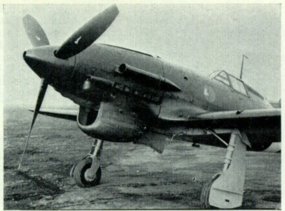
Close-up MM7768 showing the experimental chin radiator.
