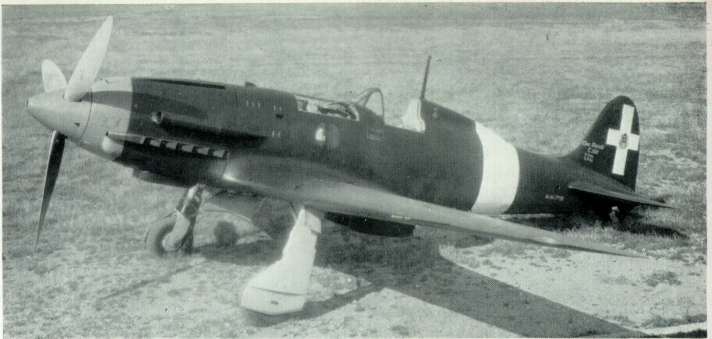
Four guns were installed in MM7731, finished dark green upper surfaces with a yellow nose band.
