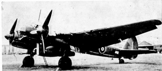
Left: Luftwaffe aircrew await the order to "mount" their Ju 88A-4. Right: This captured Ju 88A-6U reconnaissance aircraft displays search radar antennae on the wing leading edge. The ventral gondola has been omitted and long-range fuel tanks are fitted under the wing roots.
