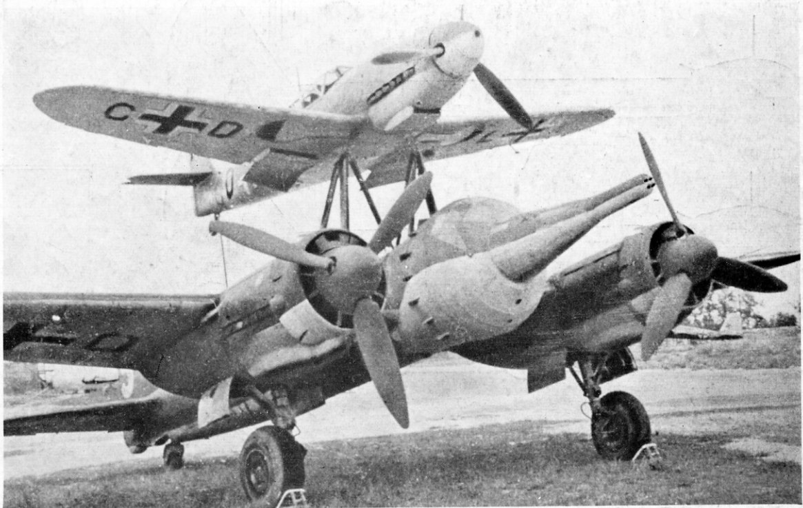
Converted Ju 88A-4's carried a 7,726-lb. hollow charge warhead as the lower component of the Gerat Beethoven/Mistel 2 composite weapon. The machine, illustrated here, was guided onto target by the Bf 109F mounted on the framework above the centre-section. Note the protruding detonators in the nose-probe.
