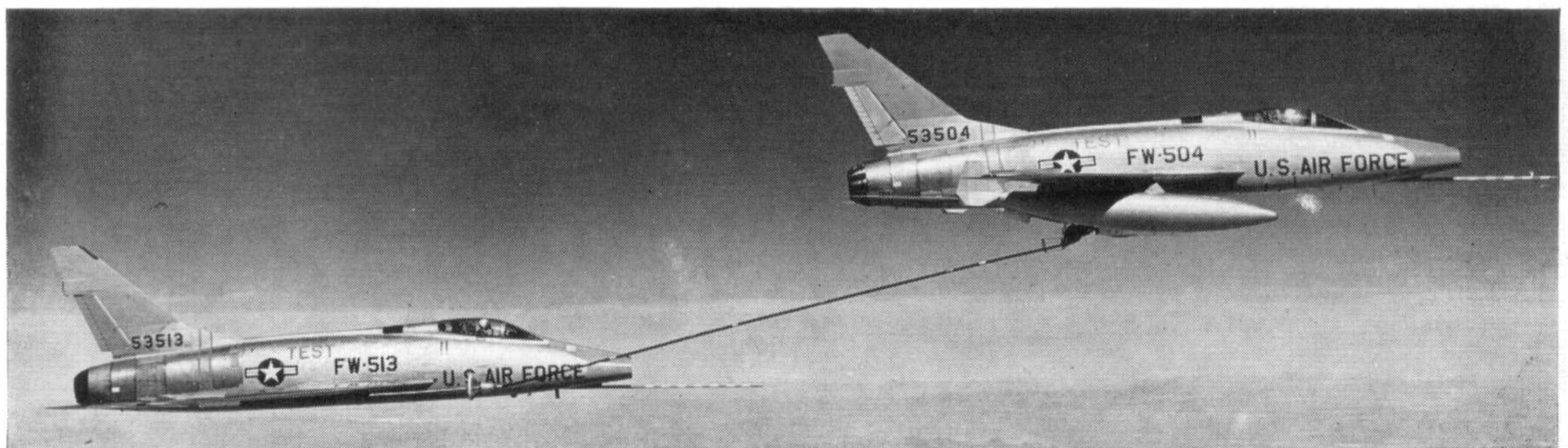
Test TF-100C which was modified from an F-100C-20. Below: F-100D-20s on a 'Buddy' flight refuelling sortie
