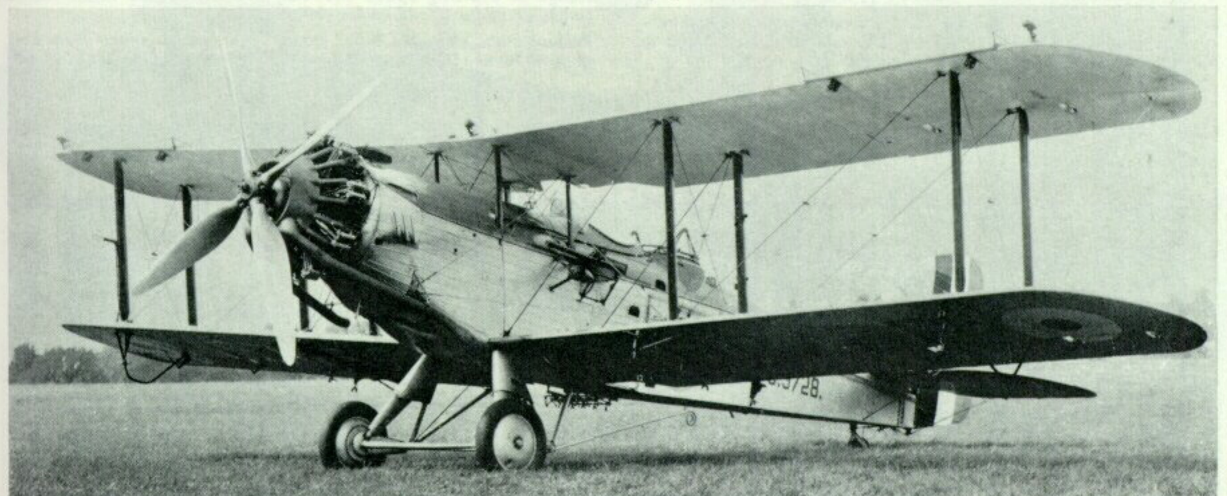
Wapiti V with Bristol Draco direct injection engine and Bristol magnesium four-blade propeller. The engine down-draught air intake is located behind top cylinders.
