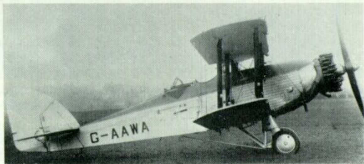
The first Wapiti V, with civil registration and A-S Panther engine, as demonstrated by Mr. Harald Penrose for the Westland Aircraft Company in South America in 1931.
