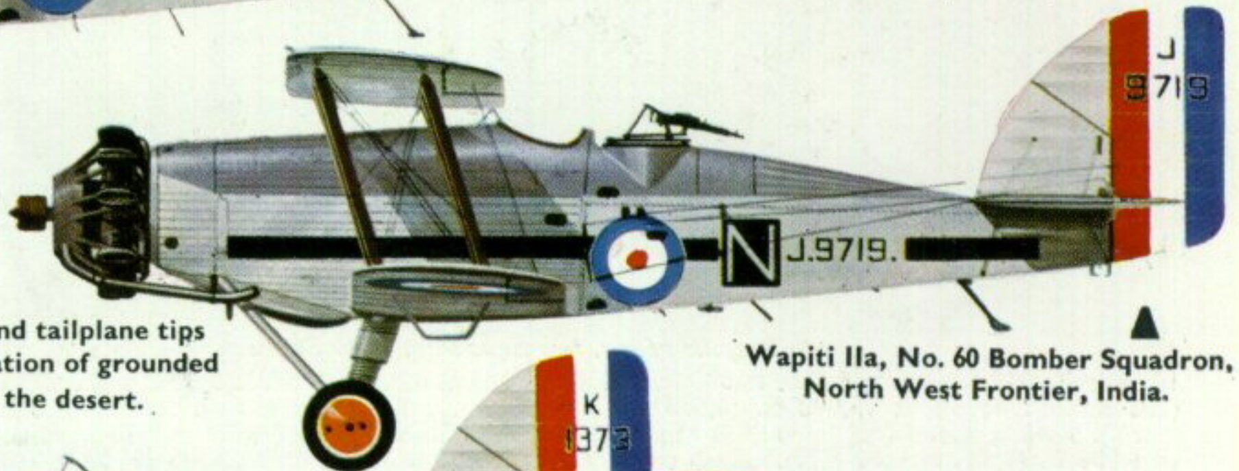
Red wing and tailplane tips for easy location of grounded a/c in the desert.
