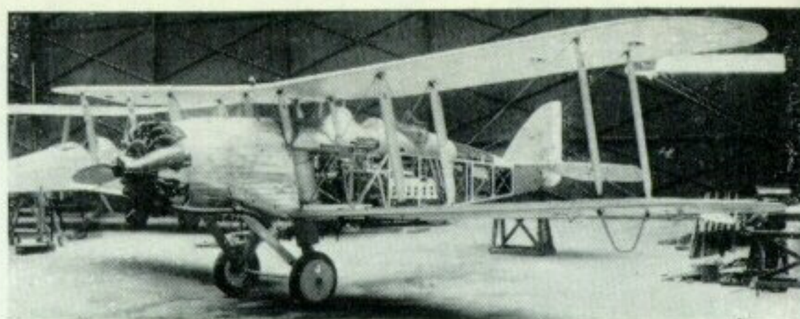
The prototype Wapiti with D.H.9A-type wings and tail.
