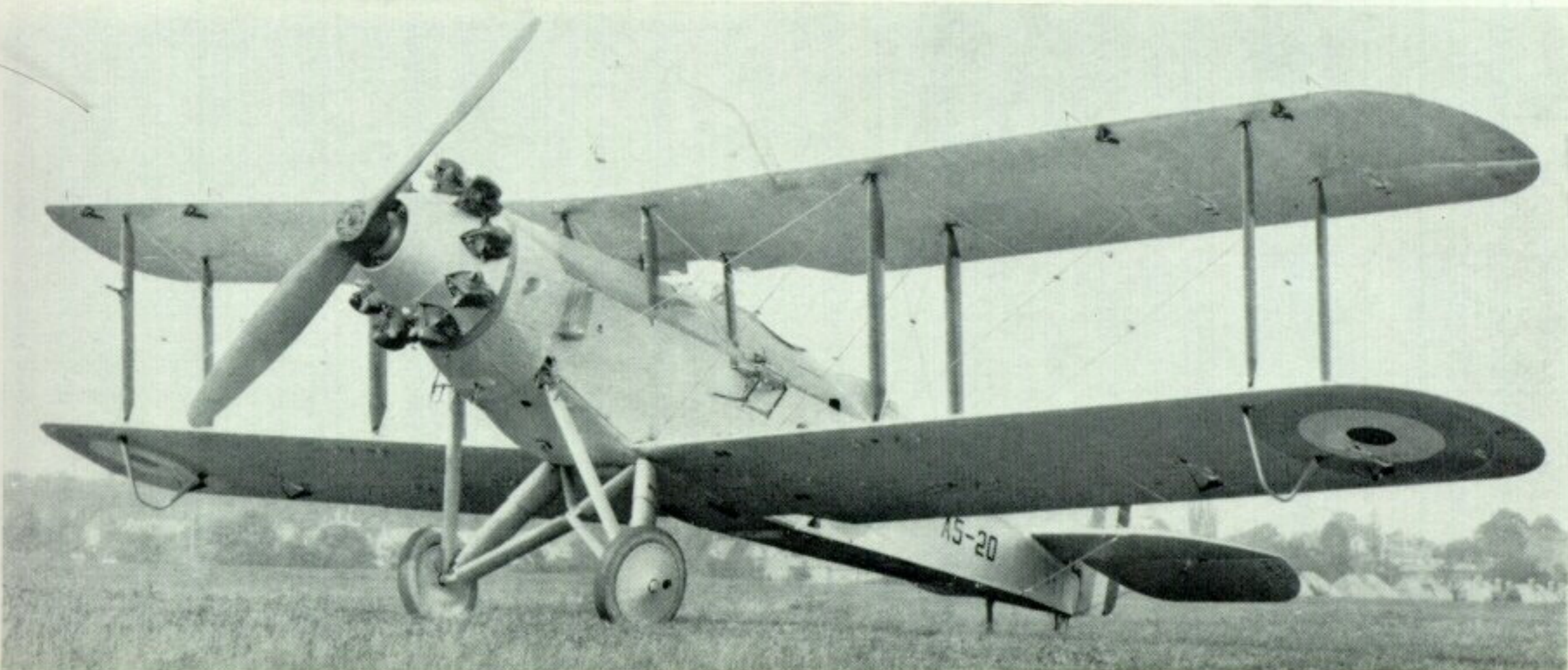
Wapiti IA for the Royal Australian Air Force with Jupiter VIII and "split axle" undercarriage.
