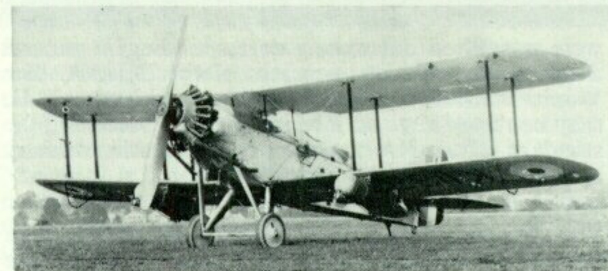
Wapiti IIA fitted with long-range underwing tanks and Jupiter IXF with distinctive exhaust collector ring. The latter was standardised on R.A.F. Wapitis of later vintage.
