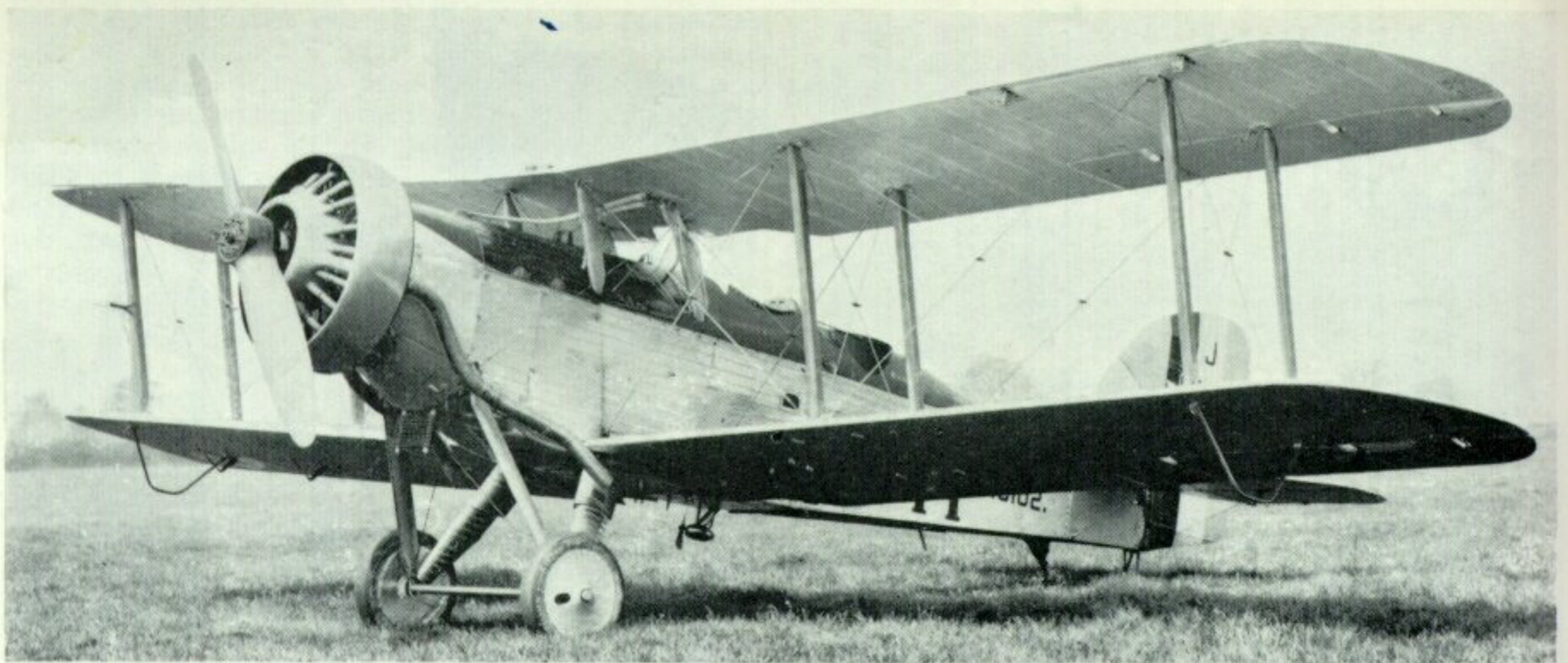
Wapiti with Bristol Phoenix diesel engine and Townend drag-reducing cowling ring as used for high altitude research.
