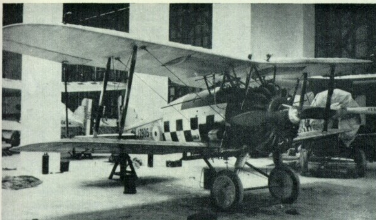
Gamecock J7905 of No. 43 Squadron with night flying equipment and Aldis gunsight. J7904 in background displays chequered top fuselage decking and flight leader's chequered pennants.
