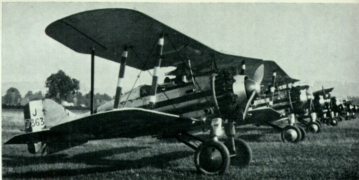
Gloster Grebes of No. 25 (Fighter) Squadron lined up at the manufacturer's Brockworth airfield. Powered by a Jaguar engine, the Grebe represented the design transition from the wartime fighting scout concept to the pure interceptor.
