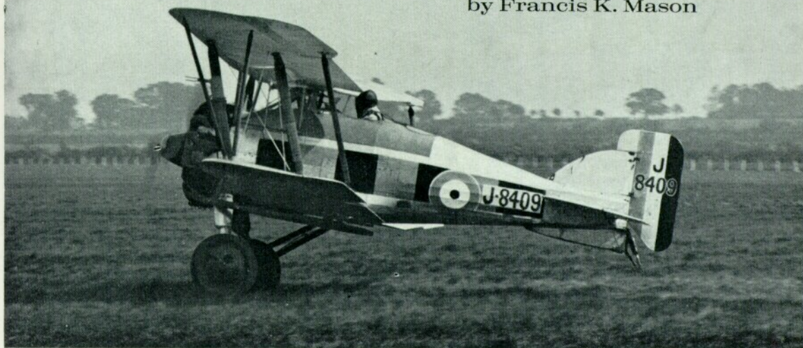
Gamecock of No. 23 (Fighter) Squadron taking off at Northolt during the Sassoon Cup competition in May, 1929. Most squadron Gamecocks had by this time acquired the extra Vee-interplane struts. (Photo: "Flight")
