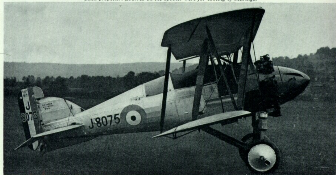
Below and on facing page: Another experimental Gamecock was J8075, used in 1929 for flight trials of the Hele-Shaw variable-pitch propeller. Louvres on the spinner were for cooling of bearings.
