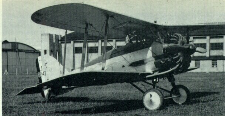
Two views of the experimental Gamecock III J8047 at an early stage in its career (August 1928) showing parallel-chord ailerons, lengthened fuselage and enlarged fin. (Photos: "Flight")
