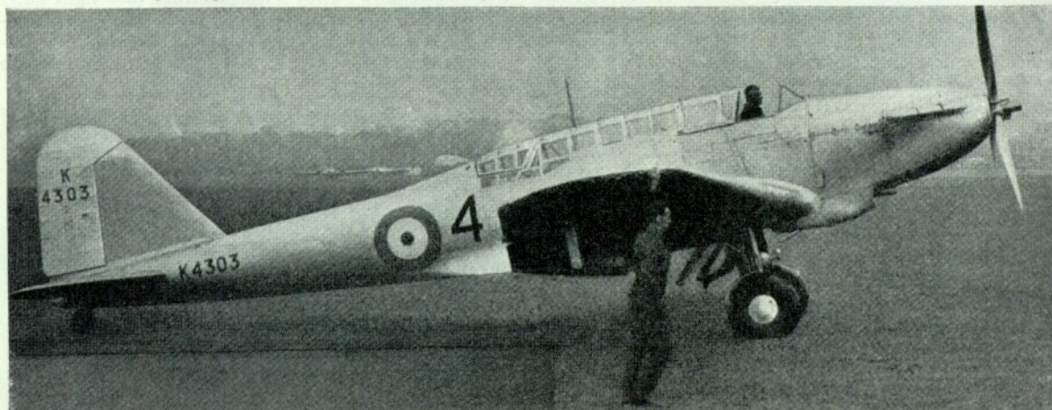
Battle prototype K4303 at the 1936 R.A.F. Display with revised cockpit canopy adopted on production a/c.
