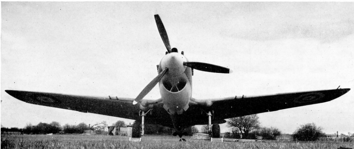
Head-on view of R.A.F. Tomahawk IIB reveals radiator air intake, cooling gills and two-tone under-surface colour scheme of blue and black. (Photo: Imperial War Museum)
