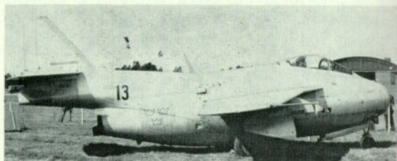
A J 29A of the F 13 Wing as used for missile tests, etc. Note fairing for observation camera under tailplane and the wing pylon.
