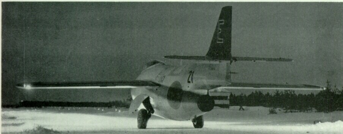
An S 29C of the F 21 Wing, Lulea. Red "E" on fin outlined in white; serial 29920. Note radar antenna under tailplane.
