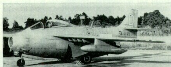
A J 29B of the F 22 Wing with drop tanks and underwing pylons.
