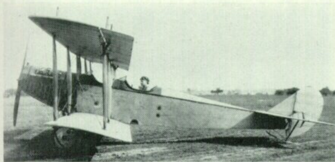
Prototype American Curtiss JN-4. Tail is virtually identical to JN-3, but was modified on production versions.
