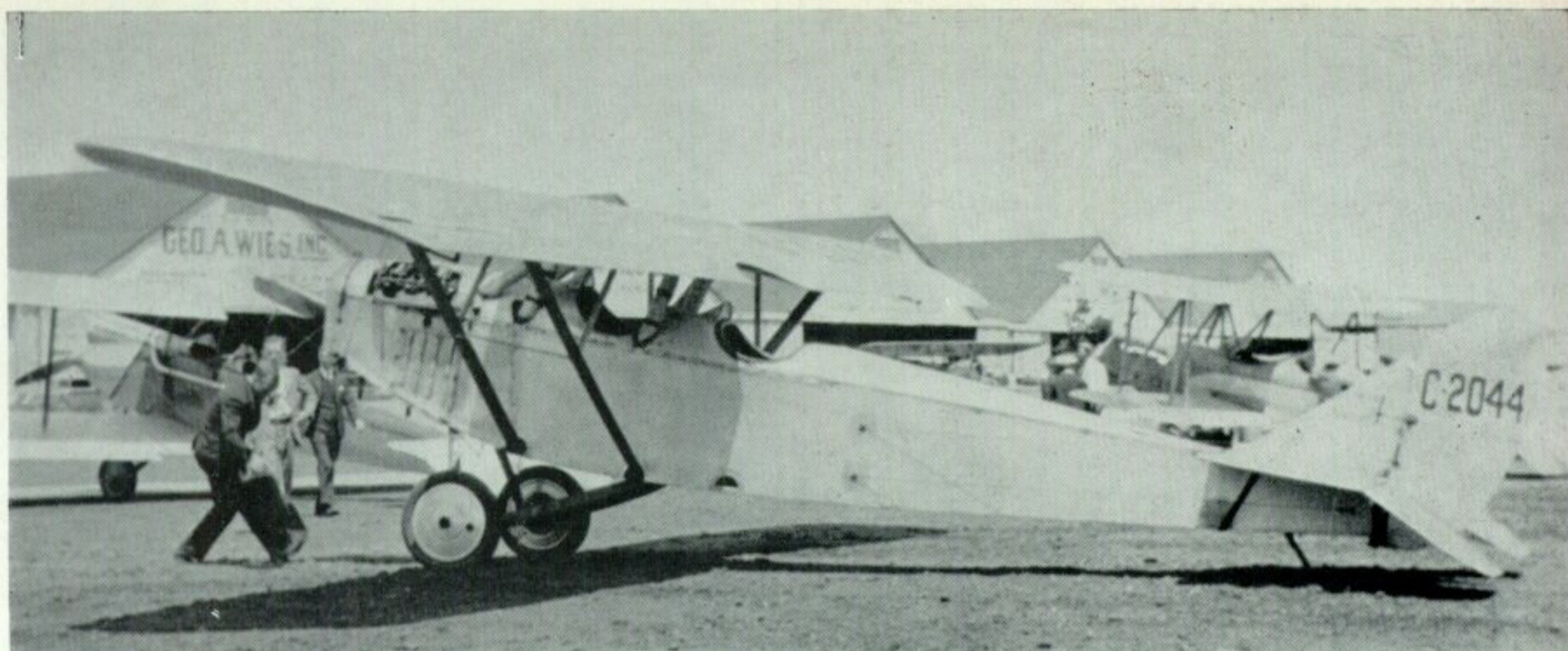
A JN-4D fitted with a monoplane wing built by Sikorsky. Several small firms developed improved wing designs for the war-surplus Jennies and Canucks.
