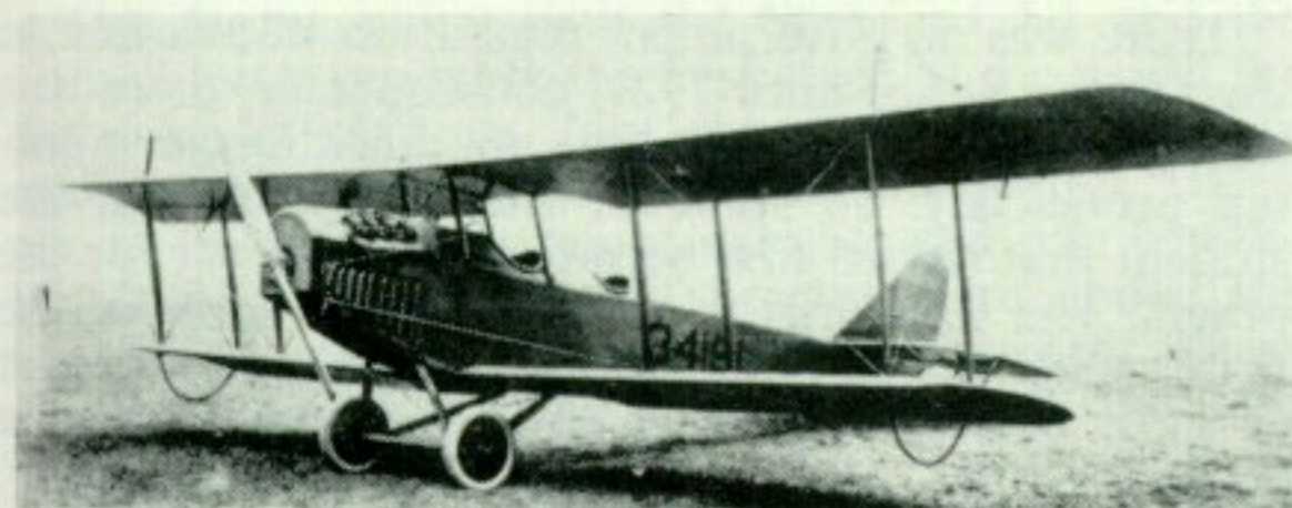
The single JN-4D-2 prototype built by Curtiss had the engine downthrust of the standard JN-4D model. Khaki-brown colouring adopted for trainers late in 1918.
