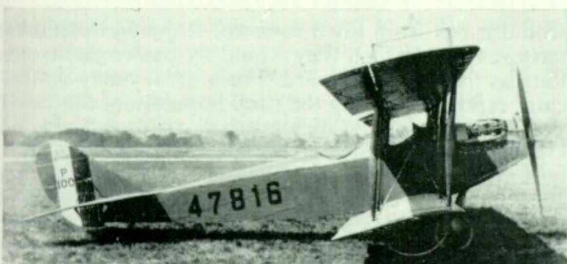
One of 100 JN-4D-2s built by Liberty Iron Works, identical to Curtiss-built prototype except for elimination of the engine downthrust.
