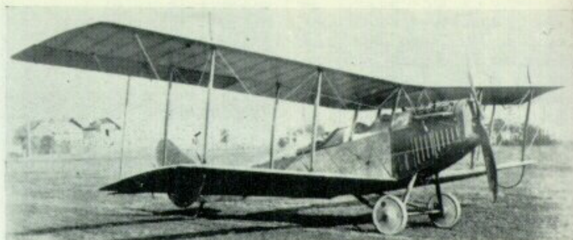
JN-4A was distinguished by new vertical tail shape and increased dihedral angle of wings.
