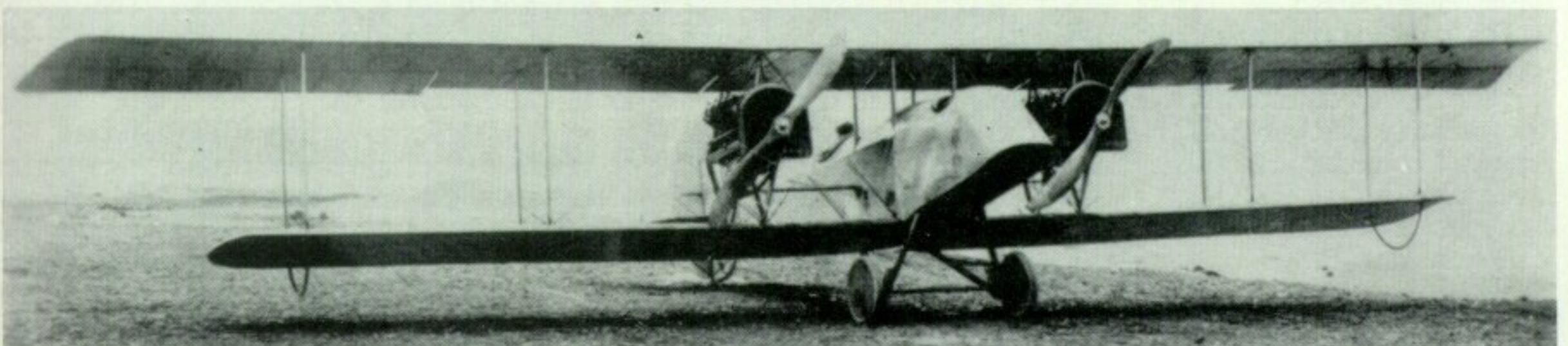
Twin JN used JN-4 wing panels and engines on a modified fuselage. Starboard engine modified to turn opposite to port engine to neutralise propeller torque in flight.
