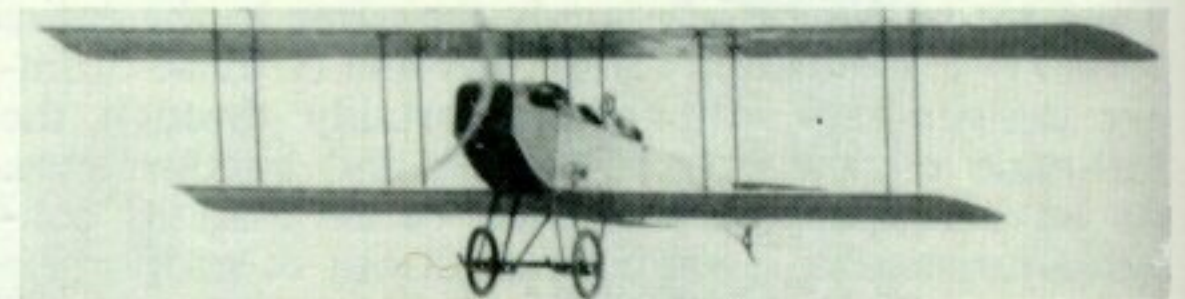
The "JN", created by combining the better features of the "J" and "N" models.
