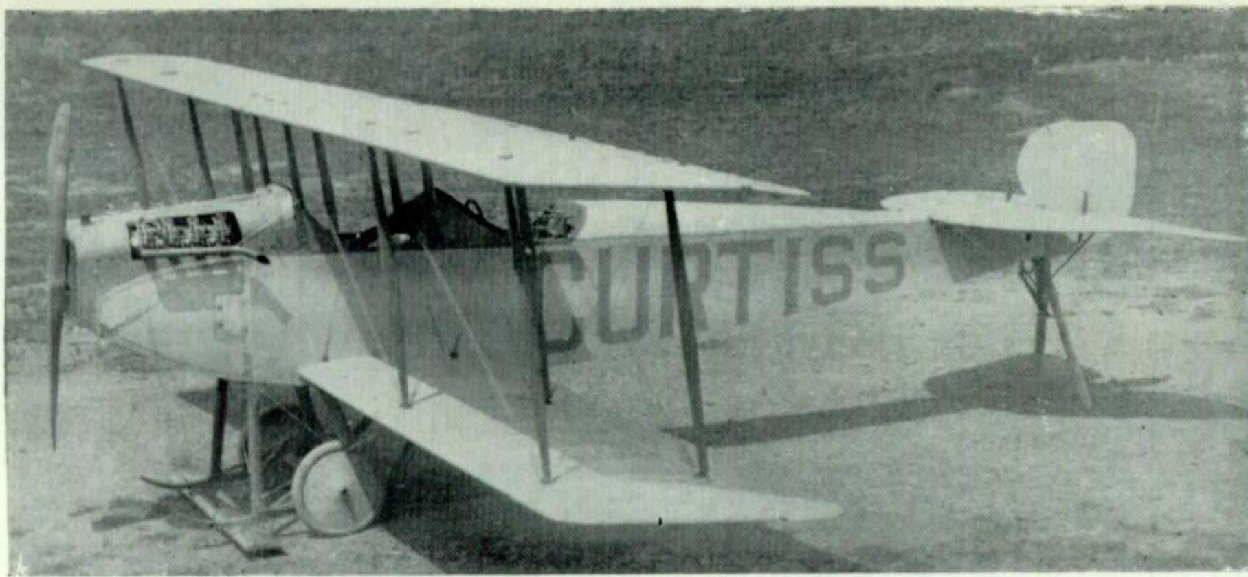
The Curtiss Model "J" in completed form. Its initial flights had been made without fabric covering on the fuselage.
