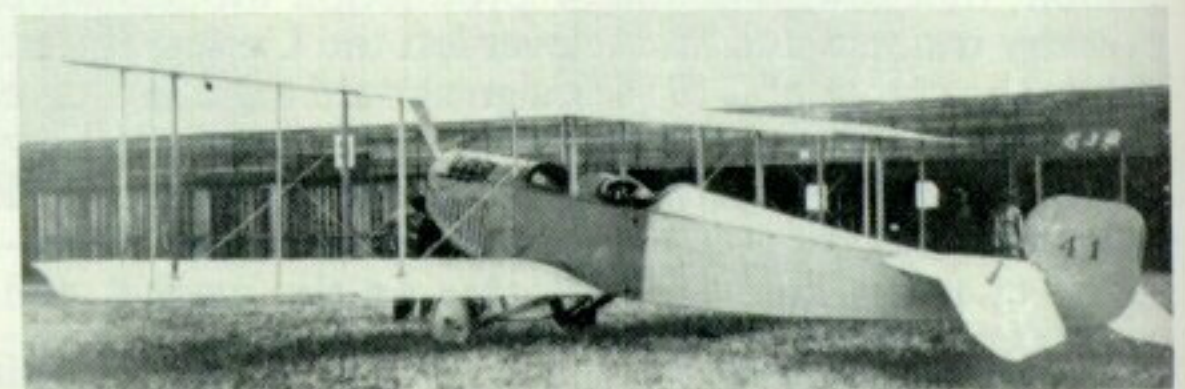
Ten JN-2s were built with this long-wing pattern. The second machine had a shorter lower wing on the pattern of the JN.
