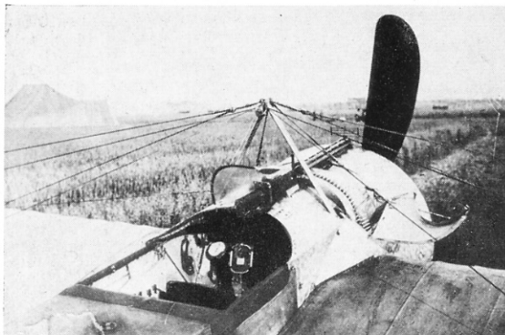
The forward fuselage of the prototype Fokker M.14, which was armed with a Parabellum gun.
