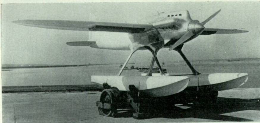
The S.4 contender for the 1925 Contest showing its cantilever construction.
