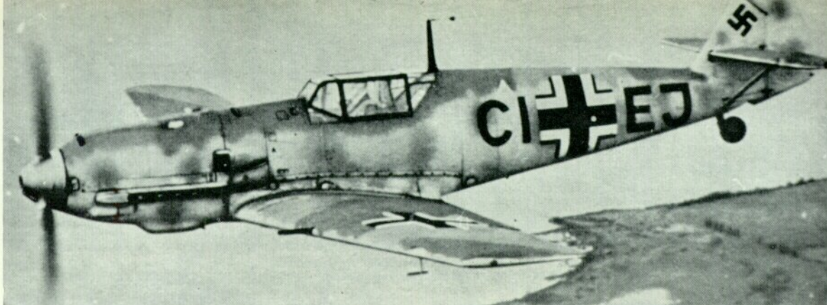
A Bf 109E-4 during flight trials displays standard 1941 colour scheme with radio call-sign codes. Note the flat-topped cockpit canopy, which offered improved armour protection over the earlier style of canopy employed on the E-3 variant.
