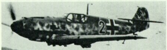
The Bf 109E-7 was essentially an improved E-4/N with shackles for a 66-imp. gal. drop tank; the variant was widely used in the Middle East. (Photo: G. Heumann/Air Pictorial)
