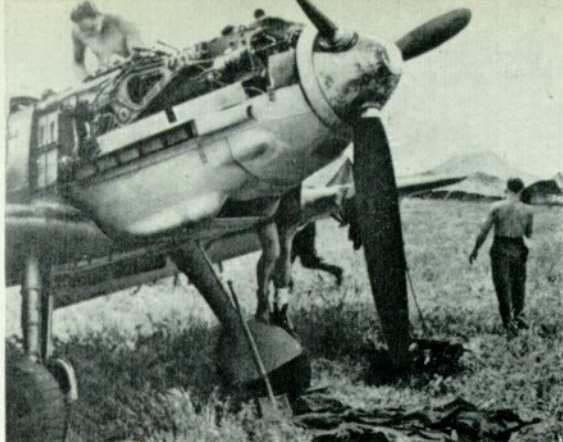
Luftwaffe mechanics at work on the DB 601N powerplant of a machine of III/JG 27 during that Gruppe's service in the Balkans. (Photo: R. Ward Collection)
