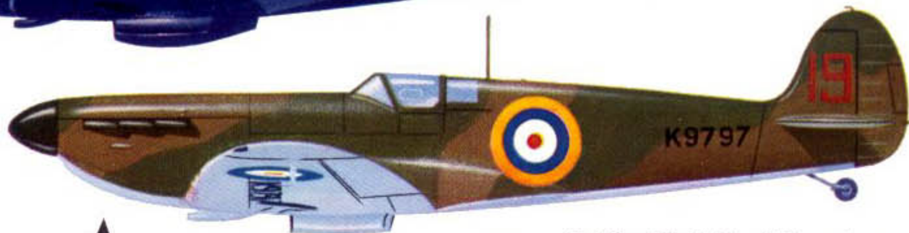
Spitfire Mk. I, No. 66 Squadron, Coltishall, U.K., 1939. Port undersurfaces black, stbd. side white or silver. Colour division was usually through the centre line of the fuselage though sometimes the wing only was black.
