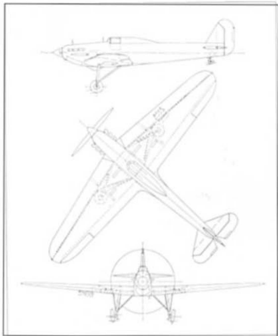
Above and below: Two of the many Supermarine F.7/30 development projects which preceded the Type 300 Spitfire. Both these projects had R-R Goshawk engines, four guns and carried four small bombs beneath the starboard wing.
