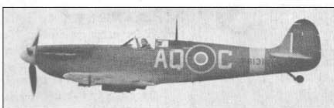
P8131, a converted Spitfire IIA, redesignated IIC. No. 276 Squadron. (Photo: "The Aeroplane")
