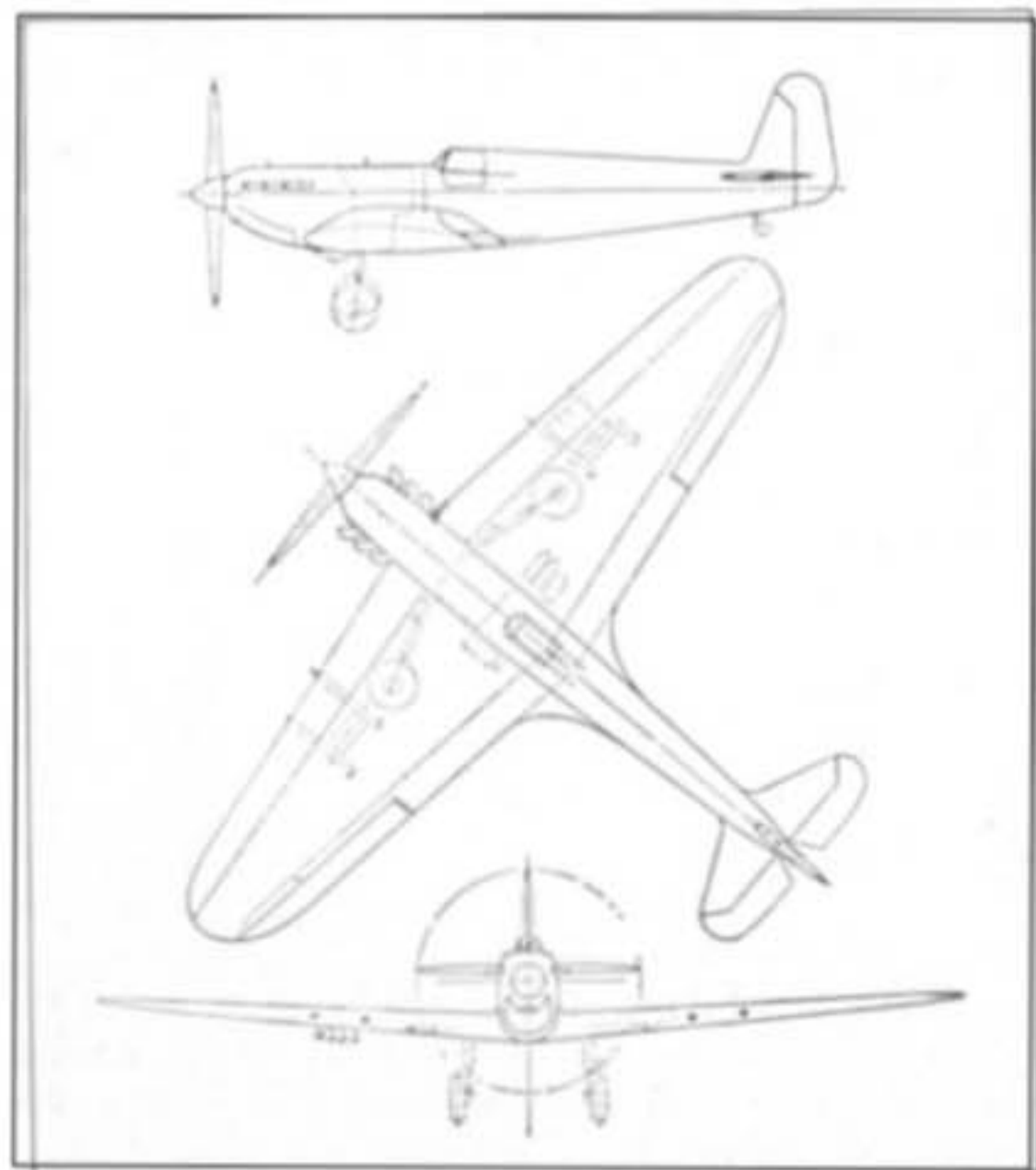
Above and below: Two of the many Supermarine F.7/30 development projects which preceded the Type 300 Spitfire. Both these projects had R-R Goshawk engines, four guns and carried four small bombs beneath the starboard wing.
