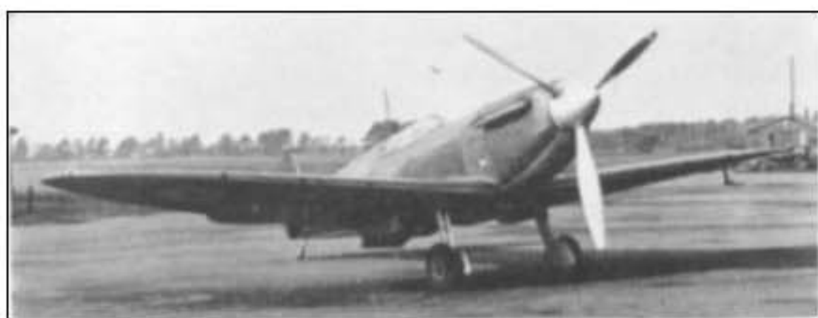
Trial installation of a de Havilland three-blade V.P. airscrew on K9793 early in 1939. (Photo: Imperial War Museum)
