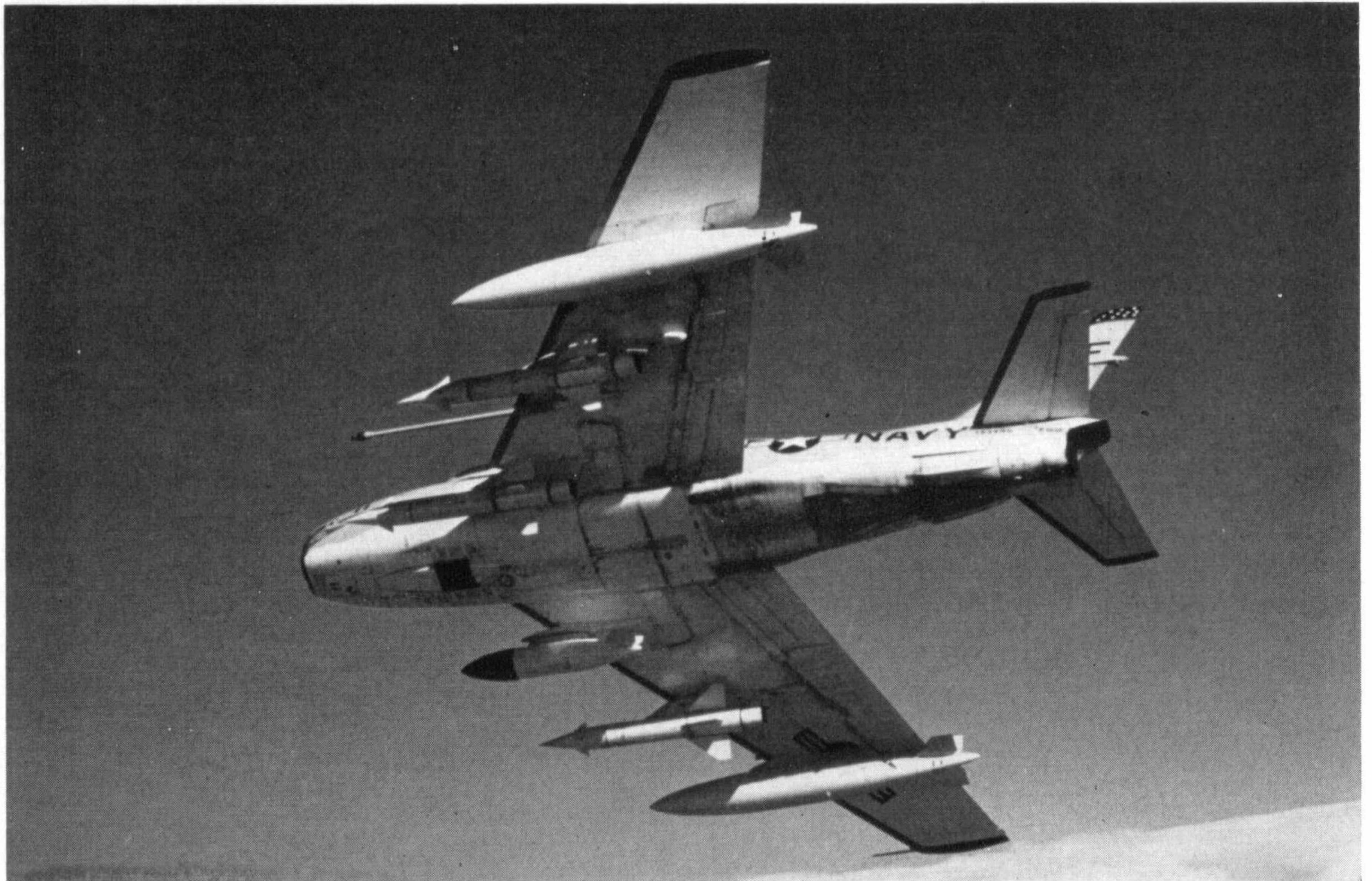
Below: Striking in-flight view of an FJ-4B with three ASM-N-7 Bullpup missiles, missile guidance pod and two drop tanks. (Photo: U.S. Navy)
