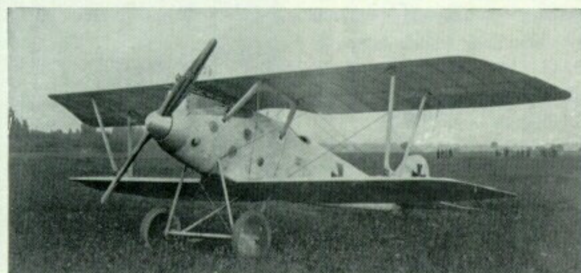
Below: Pfalz D III in mint condition shows contrast between fabric-covered aluminium-doped fuselage skin and metal of nose panelling and inspection discs. (Photo: Egon Krueger)
