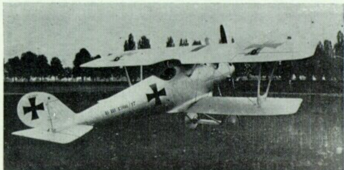
Left: Pfalz D III 4185/17 Justa 5, with red and white fuselage bands photographed at Boistrancourt. (Photo: von Hippel). Right: Early production Pfalz D III in standard ex-works aluminium finish, showing clearly style and location of patee crosses and fuselage serial number. Also to be noted—the black datum on fuselage centre-line extending back from nose. (Photo: Egon Krueger)
