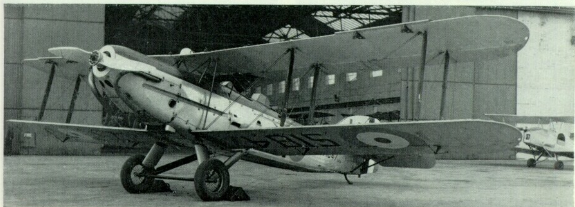
With guns omitted, S1847 was converted from IIIF Mk. III standard to IIIF (DC) standard. Seen here at Martlesham Heath, this dual-control trainer was evaluated for the Fleet Air Arm—evidenced by the jury strut necessary for wing folding. Significance of the “H” on the fin is not known but may be a relic of a previous unit. Below: S1847, frontal view. (Photos: Ministry of Defence)
