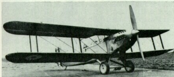
The first prototype III F, N198, as flown by Capt. Macmillan. Note the old horn-type arrester gear on the wheel axle.
