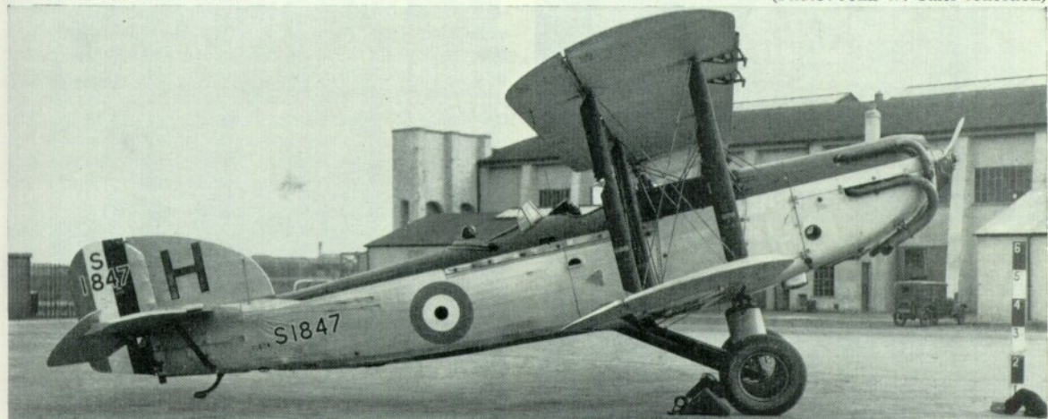
With guns omitted, S1847 was converted from IIIF Mk. III standard to IIIF (DC) standard. Seen here at Martlesham Heath, this dual-control trainer was evaluated for the Fleet Air Arm—evidenced by the jury strut necessary for wing folding. Significance of the “H” on the fin is not known but may be a relic of a previous unit. Below: S1847, frontal view. (Photos: Ministry of Defence)
