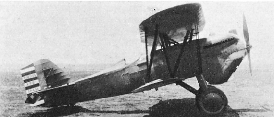
The XP-6 was a P-2 fitted with the new 600-h.p. Curtiss V-1570 "Conqueror" engine. (Photo: U.S.A.F.)
