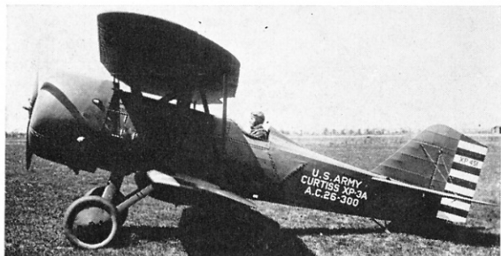
Left: The first XP-3A with the fuselage contours filled out to meet the lines of the experimental NACA engine cowling.
