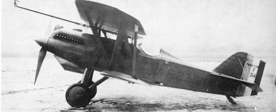
The XPW-8A became XPW-8B when fitted with new tapered wings. The long boom is part of the test equipment installed during tests at McCook Field.
