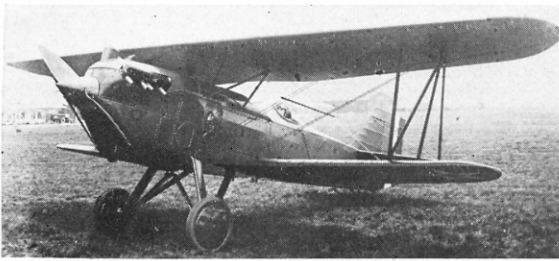
The XAT-4, a P-1A fitted with a 180-h.p. Wright-Hispano engine and tested as an advanced trainer. (Photo: Curtiss)
