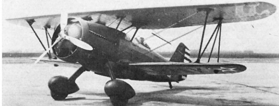
The XP-22 fitted with an experimental nose radiator during its test programme. (Photo: Curtiss)
