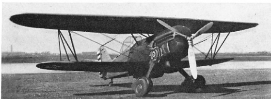
The XP-6H was the first production P-6E fitted with four wing-mounted .30 calibre machine guns in addition to the normal pair of synchronised nose guns. (Photo: D. C. Cooke)
