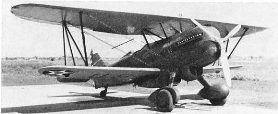
XP-6G was a standard P-6E fitted temporarily with a later model V-1570 "Conqueror" engine.
