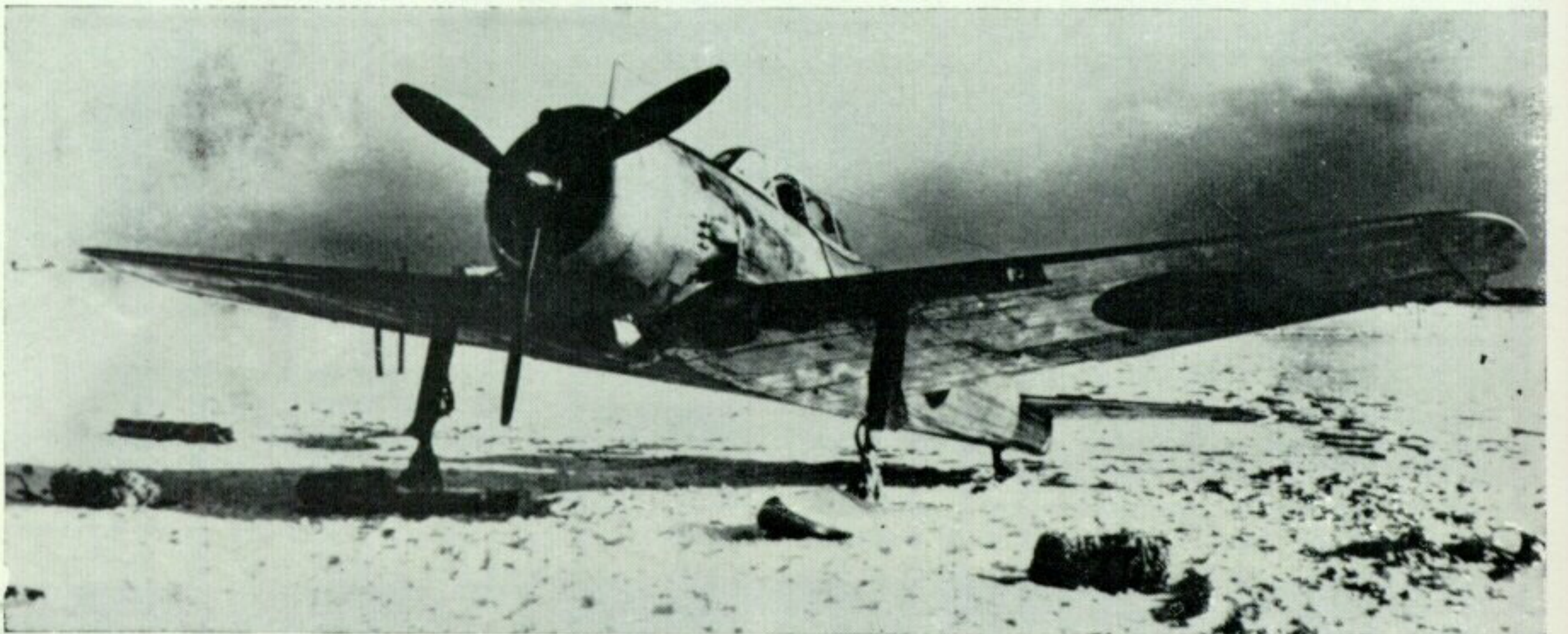
An unusual modification of the Ki-43-II KAI: a ski main undercarriage fitted for testing in Manchuria. Main gear legs were presumably locked down although this machine retains open wheel wells.
