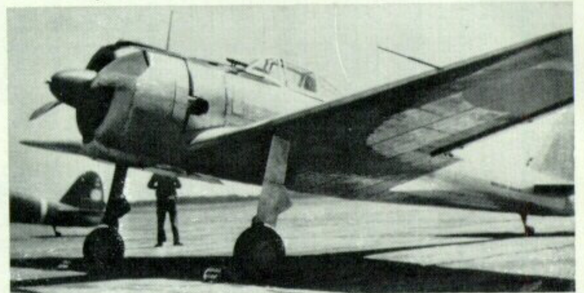
Close-up view of one of the Akeno Fighter Training School's Model 1B Hayabusas. Note airscrew decoration, fin emblem (see illustration on page 11 of this Profile) and early gunsight. (Photo: via R. J. Francillon)
