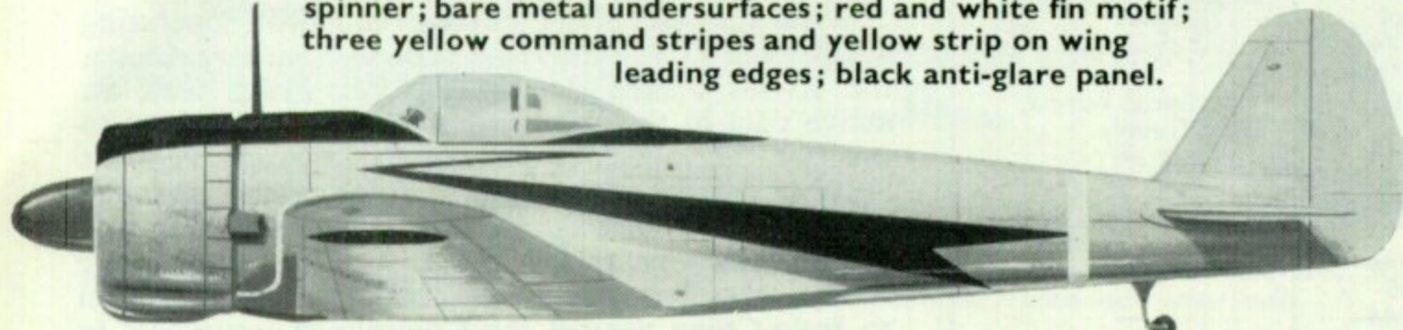
Ki-43-I, 59th Fighter Group; green spinner; black anti-glare panel; yellow strip on wing leading edges; red fuselage flash on bare metal finish.
