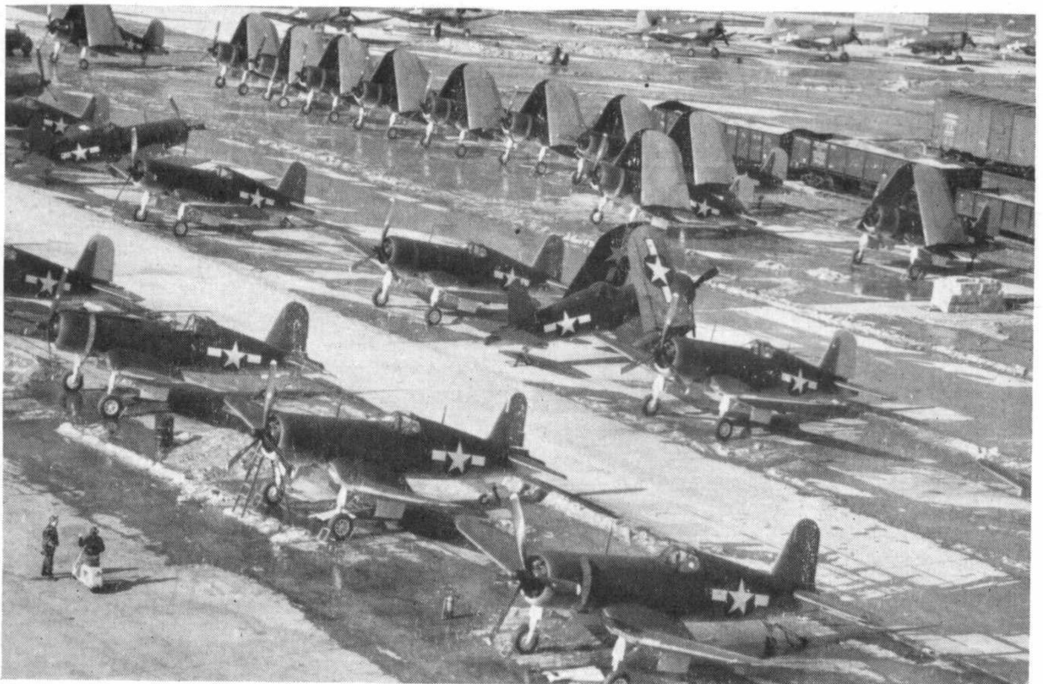
Goodyear Aircraft flight-line at the company's Akron, Ohio, plant. Note folded wings of machines in background. (Photo: Goodyear)
