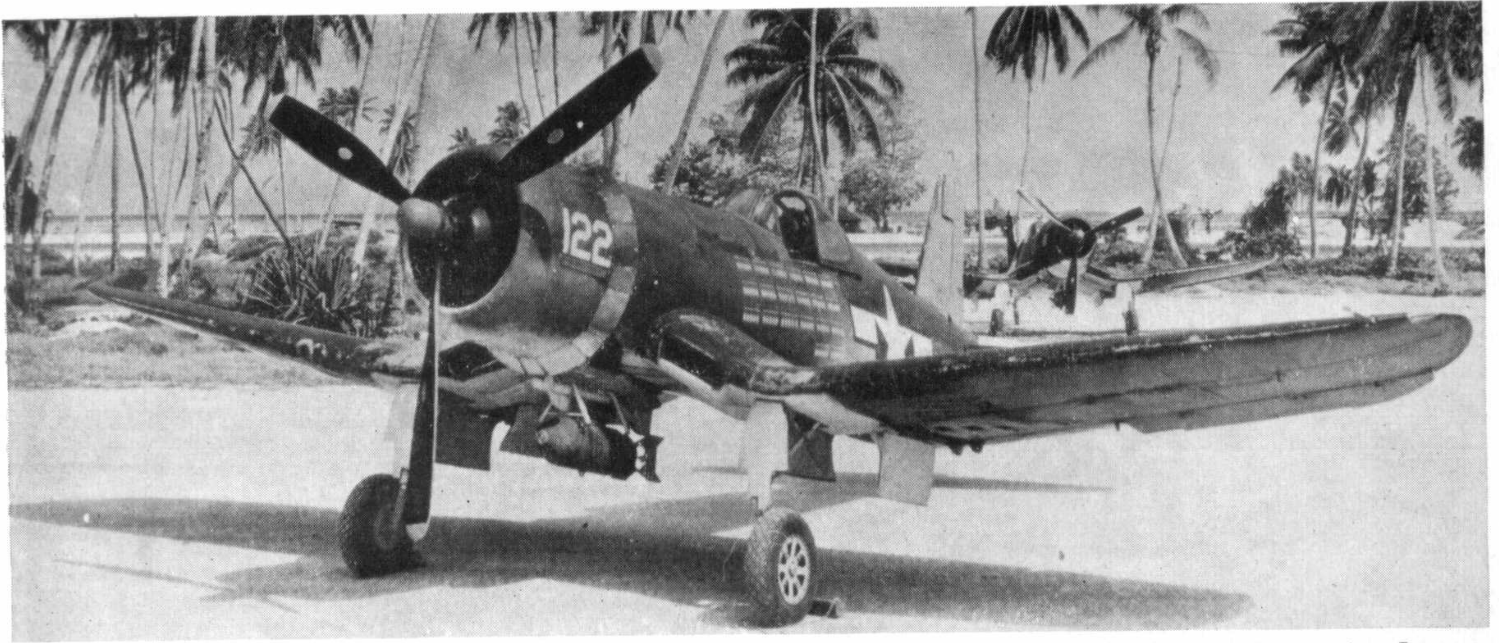
The famous "Ole 122", an F4U-1A of VMF-111 "Devil Dogs". This aircraft completed 100 dive-bombing missions against Japanese positions in the Marshall Islands, and had an official citation varnished into her cockpit. Note the 500-lb. bomb on a Brewster centre-line rack and the 100 mission markers under the cockpit. (Photo: Vought)
