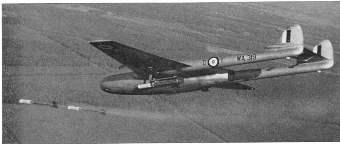
The "weathercocking" action by 3-inch rockets well demonstrated by a Vampire 5 of the 2nd Tactical Air Force during air-to-ground firing practice.
