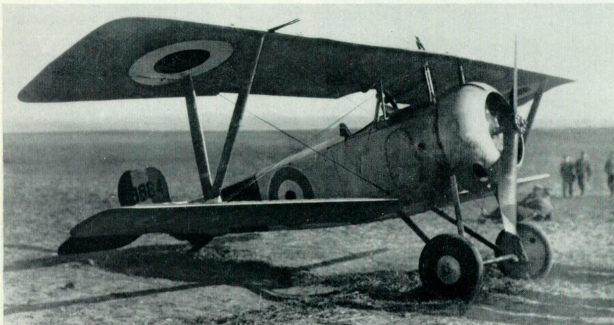
Another captured R.F.C. Nieuport 17 in German hands during the Battle of Arras, April-May 1917. Note wing-mounted pitot.
