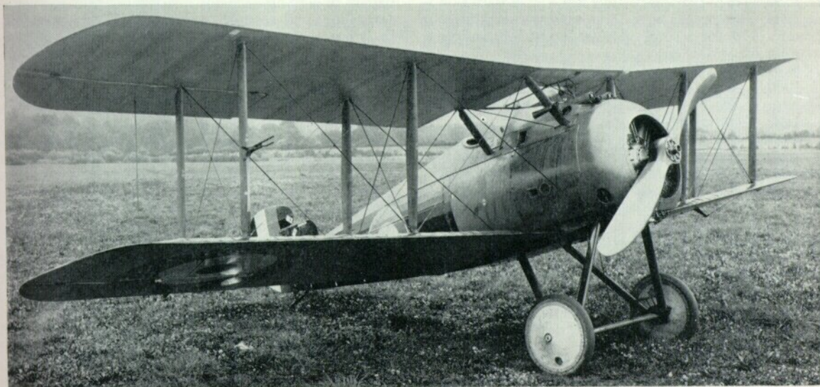
The third production Snipe built by the Sopwith company, E7989, with the first production form of fin and rudder. (Photo: Hawker Siddeley Aviation Ltd.)
