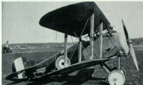
On B9966 the design of the fin and rudder was again revised and an adjustable tailplane was fitted.
