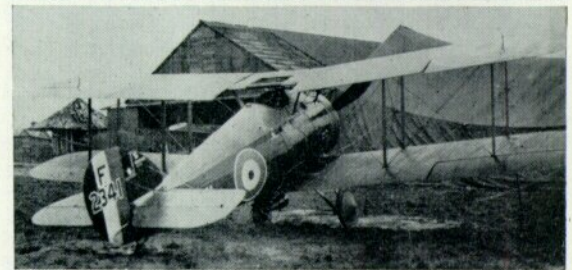
F2341 had the final form of fin and rudder but retained plain ailerons on its upper wings. The aircraft is here seen at Aulnoy, France, late in 1918, with a 112-lb. bomb under the fuselage.
