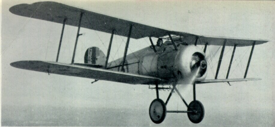
Snipe of No. 25 Squadron over Constantinople, 1923. Only the starboard Vickers gun was in place when this photograph was taken. (Photo: Ministry of Defence)
