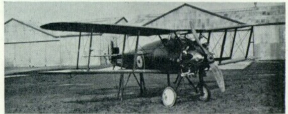
B9967 at Farnborough in March 1919 with modified Dragonfly installation. The guns had been removed by the time this photograph was made. (Photo: Crown copyright)
