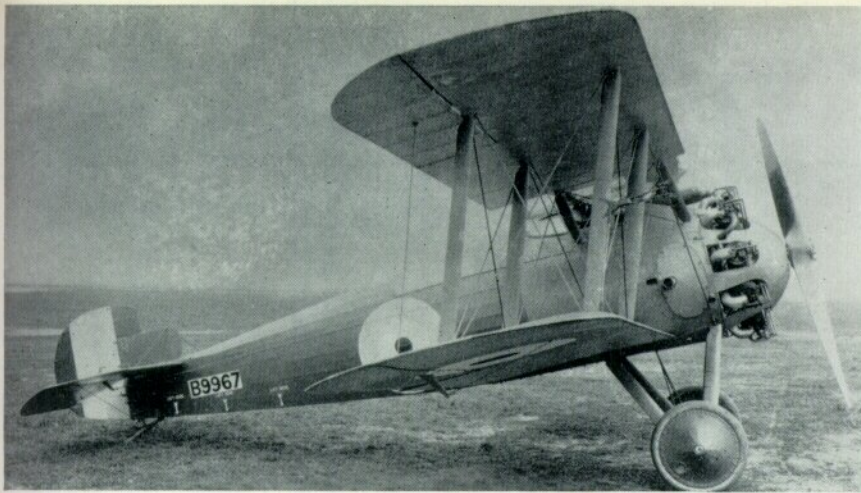
The last Snipe prototype, B9967, with 320-h.p. A.B.C. Dragonfly I engine and lengthened fuselage.
