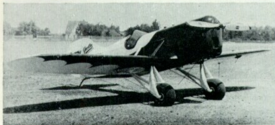
Left: The original Gee Bee Model "X" of 1930 with inverted Cirrus engine. Note that the landing gear is rigid and that flying wires are attached to the ends of the wheel axles. All shock absorbing is accomplished by the fat Goodyear airwheels. Right: Gee Bee Model "E", radial-engined version of the original "X". Flying wires now attached to a point behind the wheels, which are mounted on shock absorbers.
