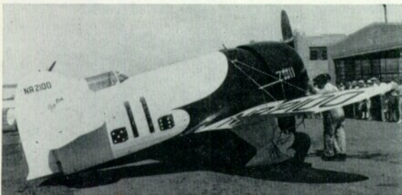
Left: The R-1 at Cleveland Municipal Airport for the 1932 National Air Races, where it won the Thompson Trophy Race and set a new Shell Speed dash record of 296.287 m.p.h. (Photo: Courtesy Charles G. Mandrake.) Right: 1933 version of the R-1 with P. & W. "Hornet" engine and increased vertical tail area.
