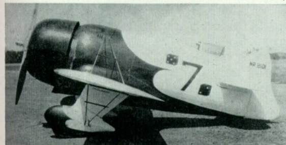
1933 version of the R-2 with engine and cowl from the 1931 version of R-1, new wing and enlarged vertical tail surfaces.
