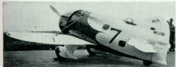
Streamlined objects above the tail registration numbers and on the wingtips of the R-2 are lights to permit night flying during cross-country races.
