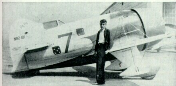
Pilot Lee Gehlbach and the Gee Bee R-2, which differed from the R-1 in having a smaller P. & W. "Wasp Jr." engine and increased tankage for cross-country racing.
