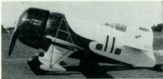
Left: The R-1 at Cleveland Municipal Airport for the 1932 National Air Races, where it won the Thompson Trophy Race and set a new Shell Speed dash record of 296.287 m.p.h. (Photo: Courtesy Charles G. Mandrake.) Right: 1933 version of the R-1 with P. & W. "Hornet" engine and increased vertical tail area.
