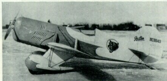
Left: Final landing gear configuration of the Gee Bee "Sportster" series. This Model "E" carries the NC lettering of a full commercial licence. Right: This Menasco-powered "Sportster" was frequently called the X-5 in spite of the fact that those aircraft with in-line engines had become known as Model "D" while those with radial engines were known as Model "E". This particular machine was raced under its commercial licence.
