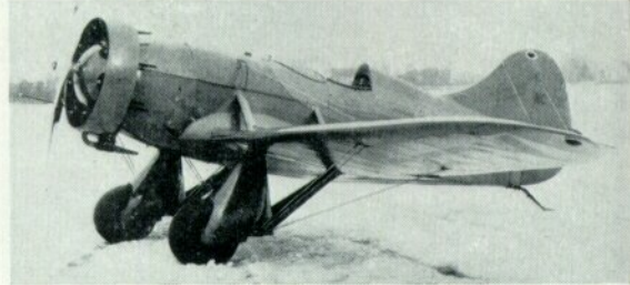
Left: The original Gee Bee Model "X" of 1930 with inverted Cirrus engine. Note that the landing gear is rigid and that flying wires are attached to the ends of the wheel axles. All shock absorbing is accomplished by the fat Goodyear airwheels. Right: Gee Bee Model "E", radial-engined version of the original "X". Flying wires now attached to a point behind the wheels, which are mounted on shock absorbers.
