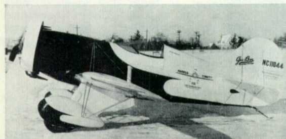
Left: Final landing gear configuration of the Gee Bee "Sportster" series. This Model "E" carries the NC lettering of a full commercial licence. Right: This Menasco-powered "Sportster" was frequently called the X-5 in spite of the fact that those aircraft with in-line engines had become known as Model "D" while those with radial engines were known as Model "E". This particular machine was raced under its commercial licence.
