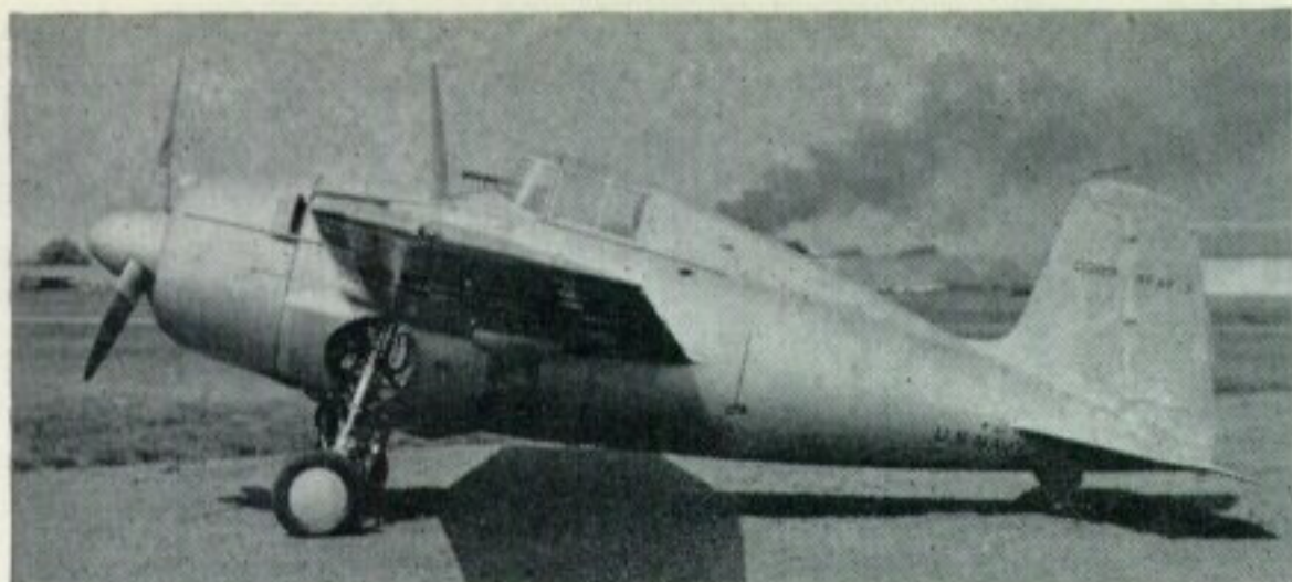
The XF4F-3 as it appeared in August 1939 with enlarged vertical tail surfaces, spinner, and cuffs on the propeller blades. (Photo: U.S. Navy)
