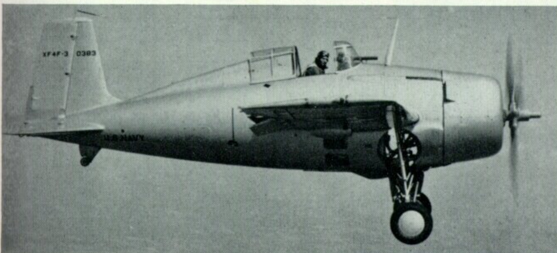
The XF4F-3 in the landing configuration, with flaps and undercarriage down.
