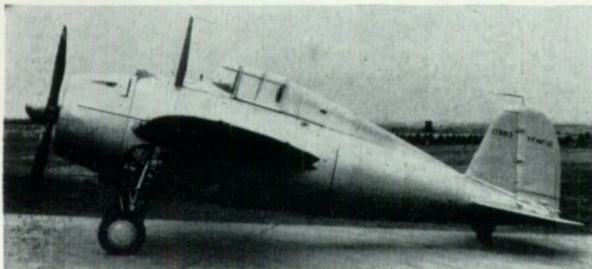
The XF4F-2 as it appeared early in 1938 with small spinner. (Photo: U.S. Navy)
