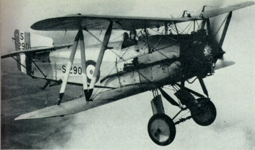
This Flycatcher, S1290 (Fairey constructor's number F 1114) was from the sixth main production batch, S1273 to S1297. Note the long exhaust pipe, not fitted to all aircraft. (Photo: Air Ministry)
