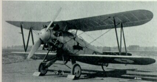
Left: Prototype Flycatcher, N163, fitted with a Bristol Jupiter engine. The early form of deck arrester gear (to engage longitudinal wires) can be seen on the undercarriage spreader bar. Right: Second version of the Flycatcher prototype with an Armstrong Siddeley Jaguar engine installed.
