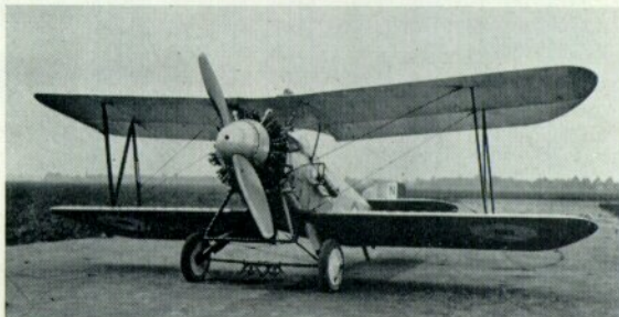
Left: Prototype Flycatcher, N163, fitted with a Bristol Jupiter engine. The early form of deck arrester gear (to engage longitudinal wires) can be seen on the undercarriage spreader bar. Right: Second version of the Flycatcher prototype with an Armstrong Siddeley Jaguar engine installed.
