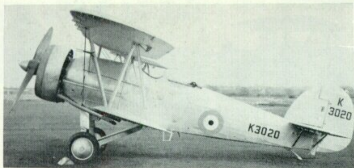
Above and below: The Bristol test-bed Hart, K3020, was flown in turn with short- and long-chord cowlings round Pegasus engines, and with Mercury driving Hamilton 3-blade metal propeller.
