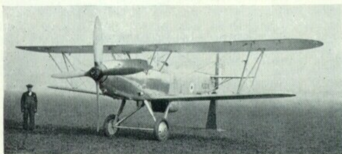
P.V.12 (Merlin prototype) installation in Hart K3036. (Photo: Hawker Aircraft Ltd.)
