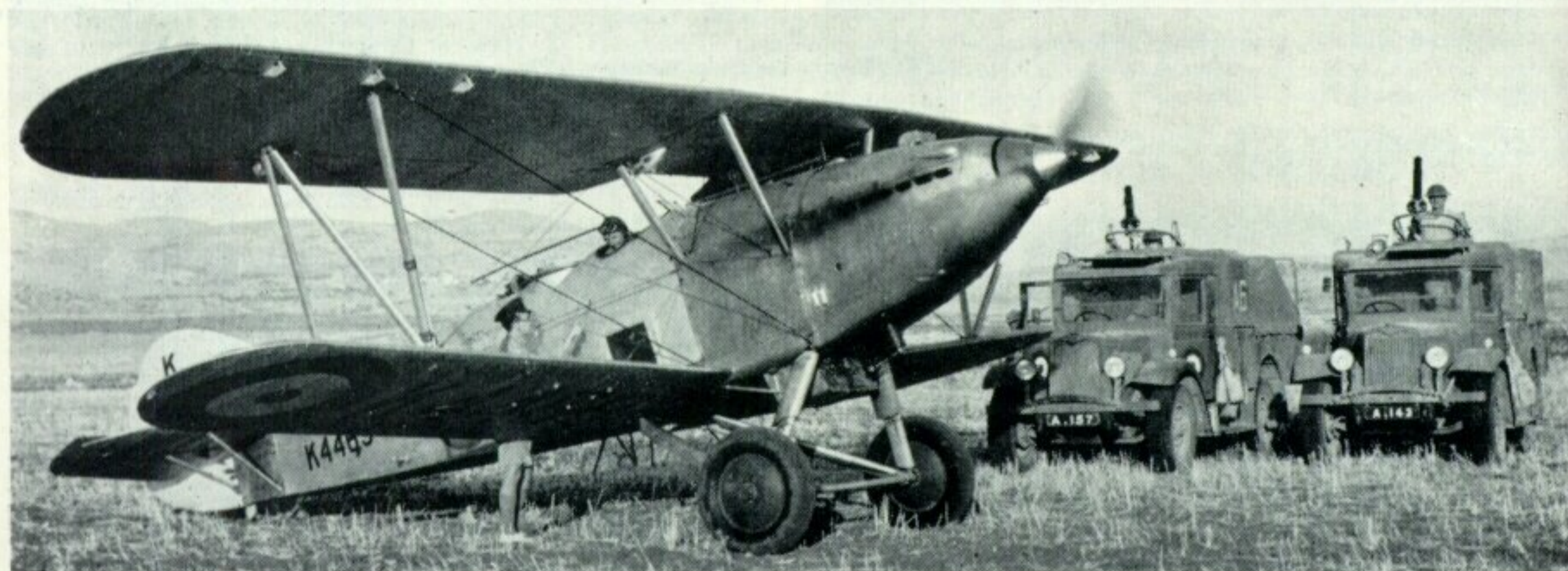
A Hart (Special), K4469, serving with the Royal Air Force in Trans-Jordan during 1940. Note the low-pressure tyres. (Photo: Ministry of Defence)
