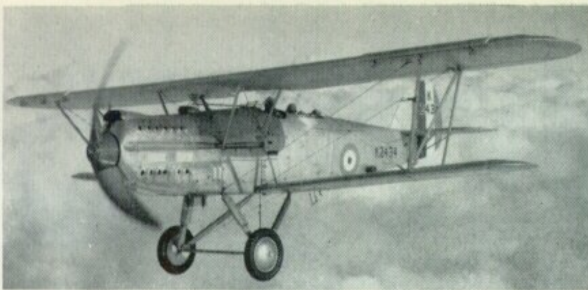
The Napier Dagger I 24-cylinder H-engine being test-flown in Hart K2434. (Photo: Flight No. 13716)
