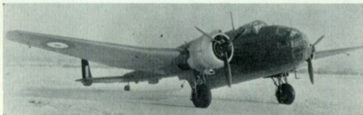
(Above and below): X3115, first of two Hampdens which were fitted with 1,100 h.p. Wright Cyclone GR1820-G105A radials. In this form they were known by the designation H.P.62 Hampden II.
