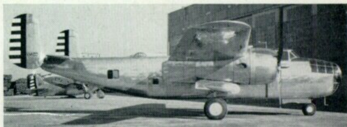
Two views of the NA-40B attack bomber, precursor of the B-25 layout. Armament for this aircraft, which crashed after passing U.S.A.A.C. trials, was envisaged as seven .30 cal. machine guns, including two fixed weapons in each wing outboard of the nacelle.
