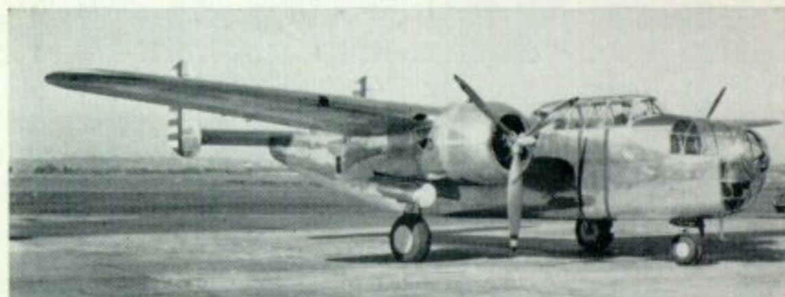
Two views of the NA-40B attack bomber, precursor of the B-25 layout. Armament for this aircraft, which crashed after passing U.S.A.A.C. trials, was envisaged as seven .30 cal. machine guns, including two fixed weapons in each wing outboard of the nacelle.
