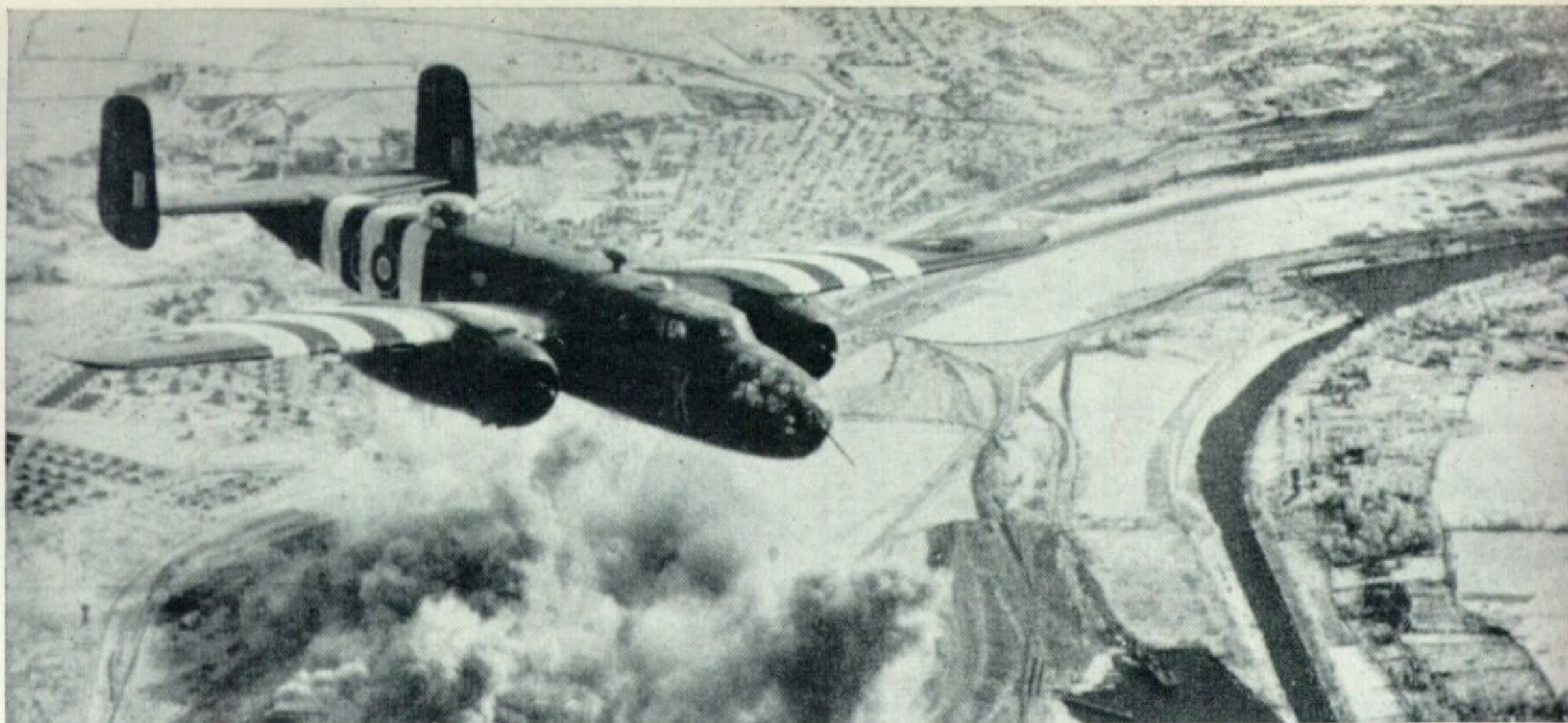
This well-known photograph of a Mitchell of No. 320 Squadron R.A.F. in action over Europe shows the D-Day invasion stripes to good effect. The machine illustrated is NO-K; note that the R.A.F. fin flashes are marked on the inner and outer vertical tail surfaces. (Photo: Imperial War Museum)
