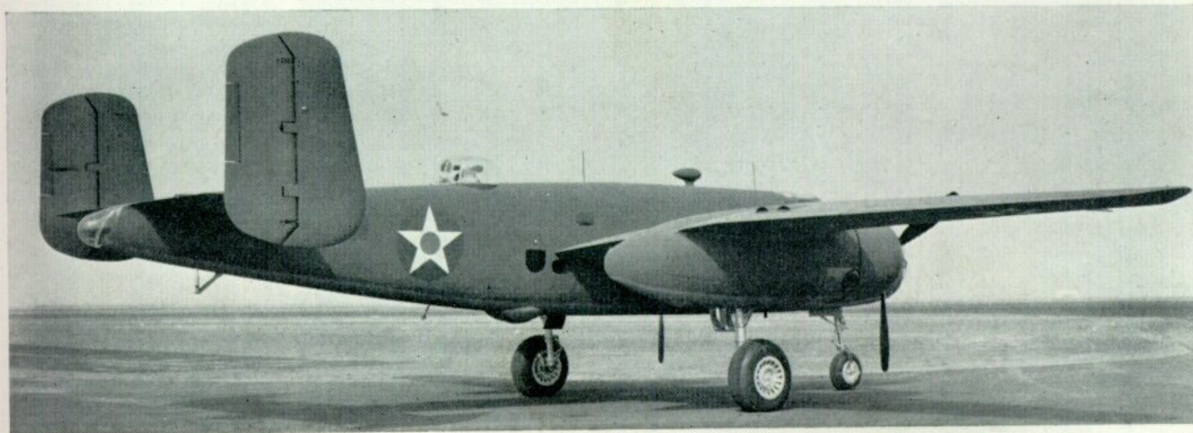
The B-25B with power-operated dorsal and retractable belly turret.
