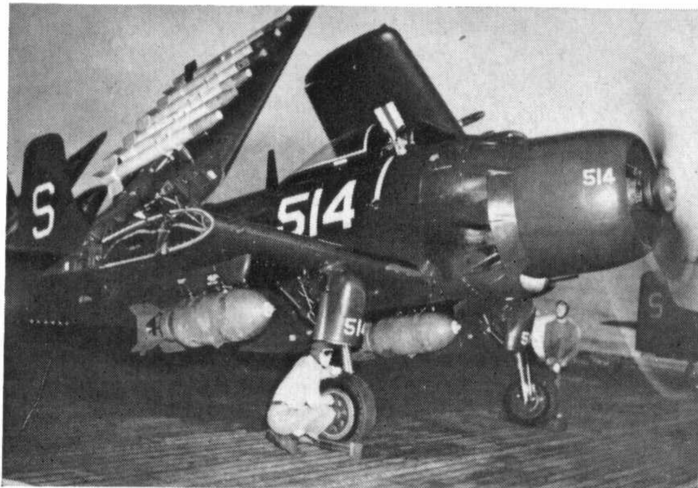
VA-55 awaits the signal to strike a target in Korea. This AD-4 is armed with twelve 5-in. rockets and two 500-lb. bombs.
