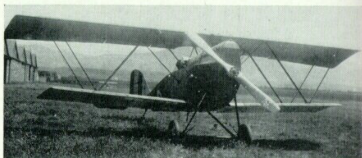
An operational S.V.A.4. Note that the starboard machine gun has been removed; this was often done when reconnaissance cameras were carried. (Photo: Col. Cesar Milani)
