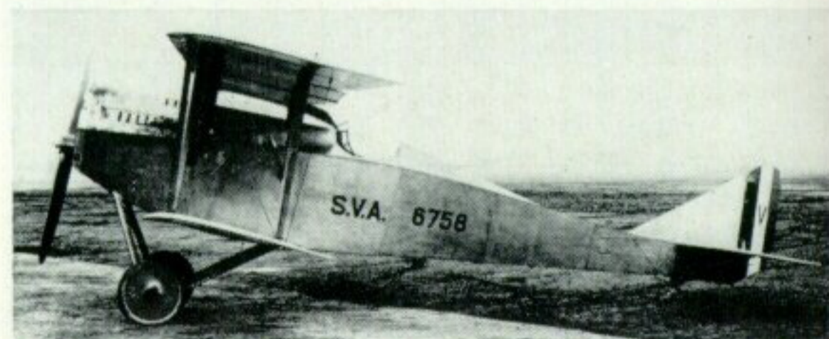
The S.V.A.5 prototype; notice the different windscreen style and the unvarnished finish. (Photo: Imperial War Museum)
