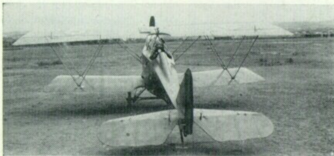
Rear and side views of the S.V.A.5: the Warren truss strut layout is very apparent, and invites immediate comparison with the Fiat biplane fighters of the 1930s.
