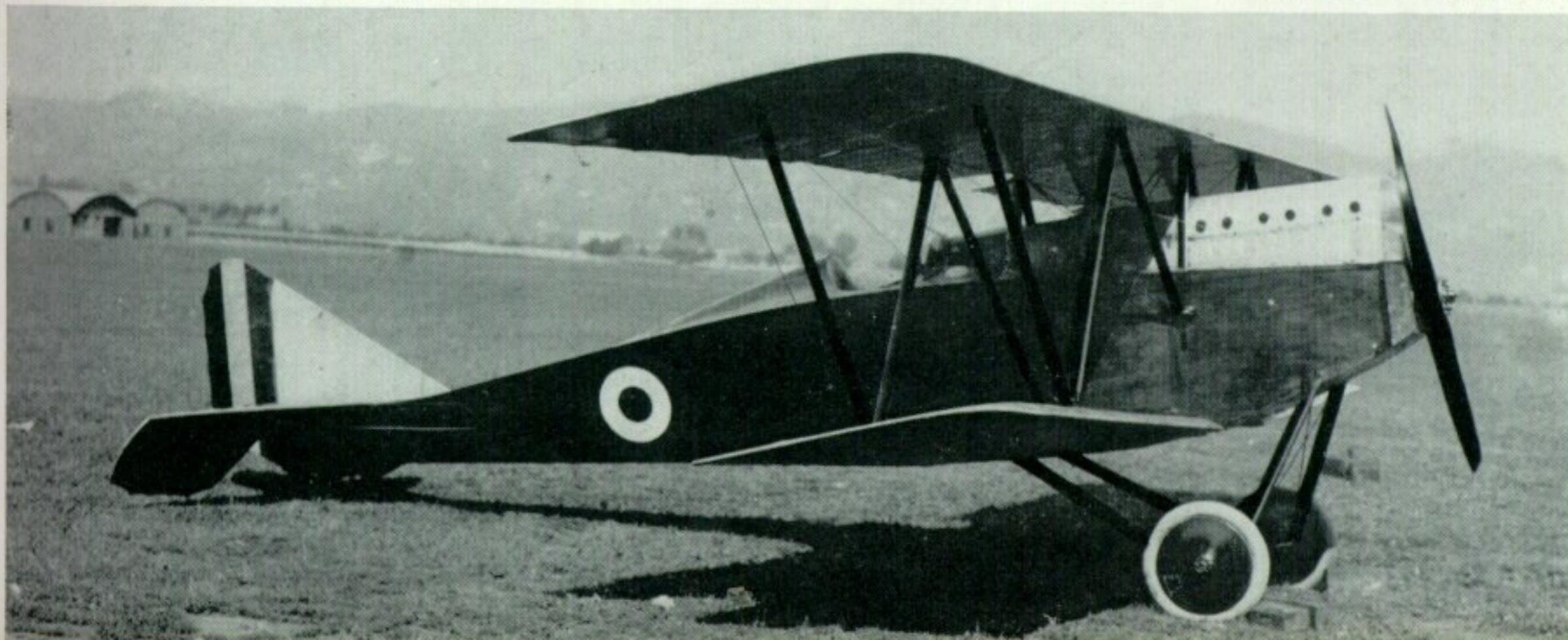
Rear and side views of the S.V.A.5: the Warren truss strut layout is very apparent, and invites immediate comparison with the Fiat biplane fighters of the 1930s.
