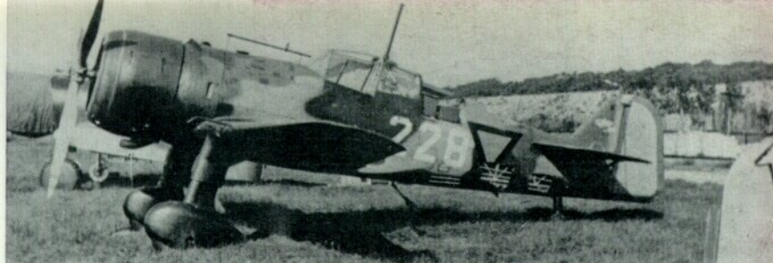
D.XXI No. 228 displays battle damage to the rear fuselage; radio and battery are exposed by the removal of the access panel. This photo was probably taken shortly after Dutch capitulation in May 1940.
