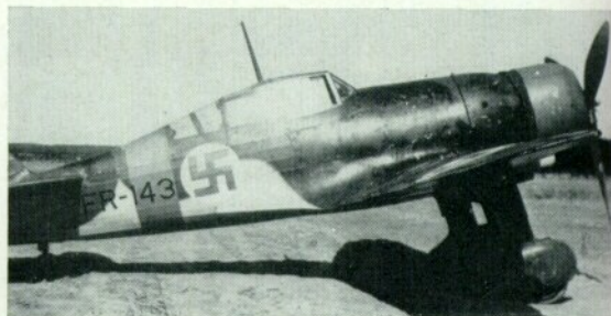
One of the modifications made by the Finnish State Aircraft Factory to the D.XXI was the rearward extension of the cockpit glazing to improve rear vision. This installation was tested on FR-143, a Mercury-engined machine.
