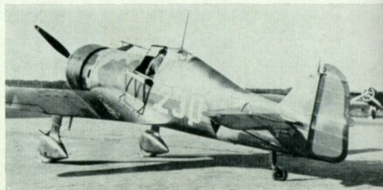
Left: FR-107, the only retractable-undercarriage D.XXI. Right: The eighteenth machine of the thirty-six ordered for the LVA. The aircraft is seen here in the national insignia adopted in October 1939; note that the wing triangle is painted well inboard. Note also the canopy section hinged fully down.
