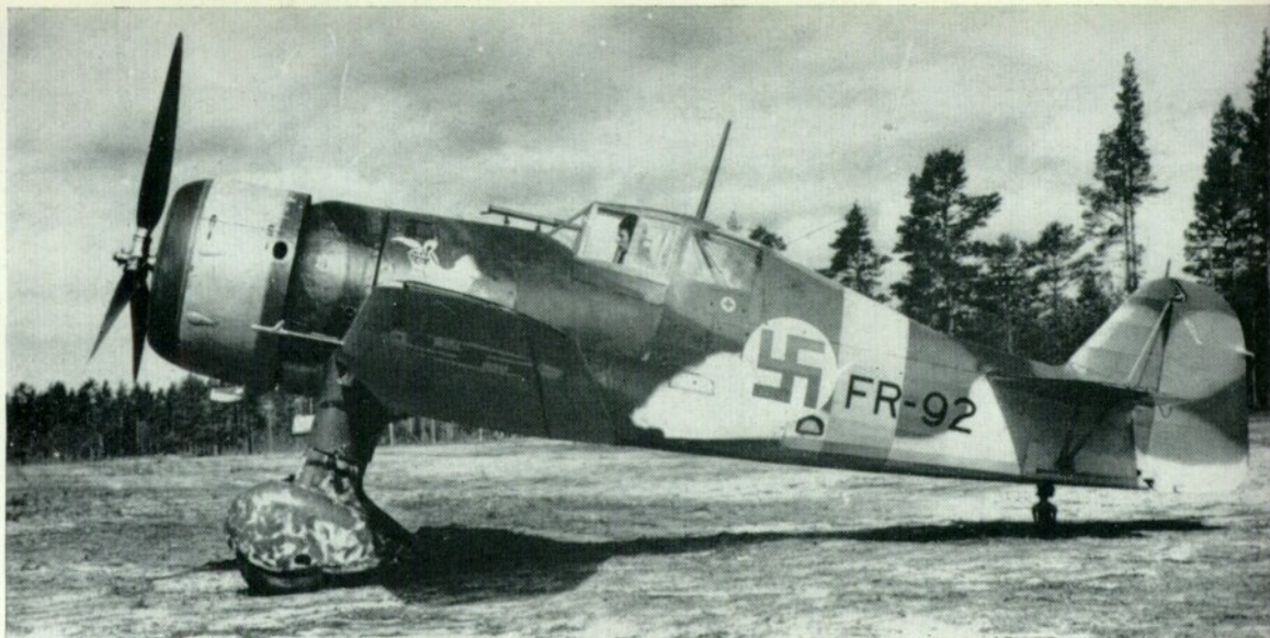
FR-92, the tenth Finnish-built D.XXI, seen here in the colourful operational markings of TLeLv. 12. The stippled effect on the undercarriage spats was thought to be deliberate decoration, but recent research indicates that it is the result of superficial damage and paint-chipping. This aircraft is the subject of the five-aspect painting on page 2 of this Profile.
