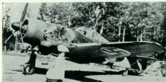
Left: FR-107, the only retractable-undercarriage D.XXI. Right: The eighteenth machine of the thirty-six ordered for the LVA. The aircraft is seen here in the national insignia adopted in October 1939; note that the wing triangle is painted well inboard. Note also the canopy section hinged fully down.
