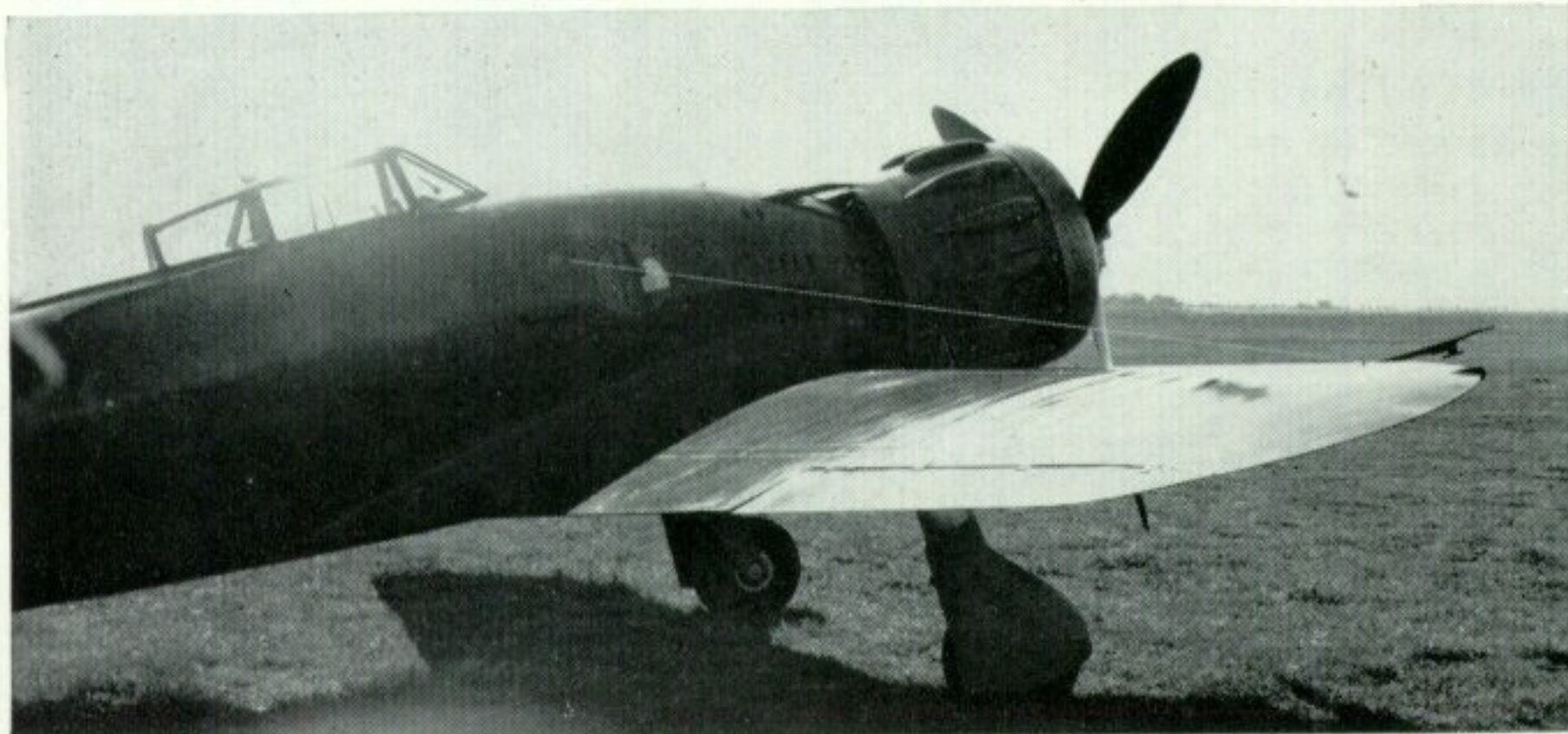
The barrels of the .5-inch SAFAT machine guns can be clearly seen protruding from the forward fuselage of this Series I machine.
