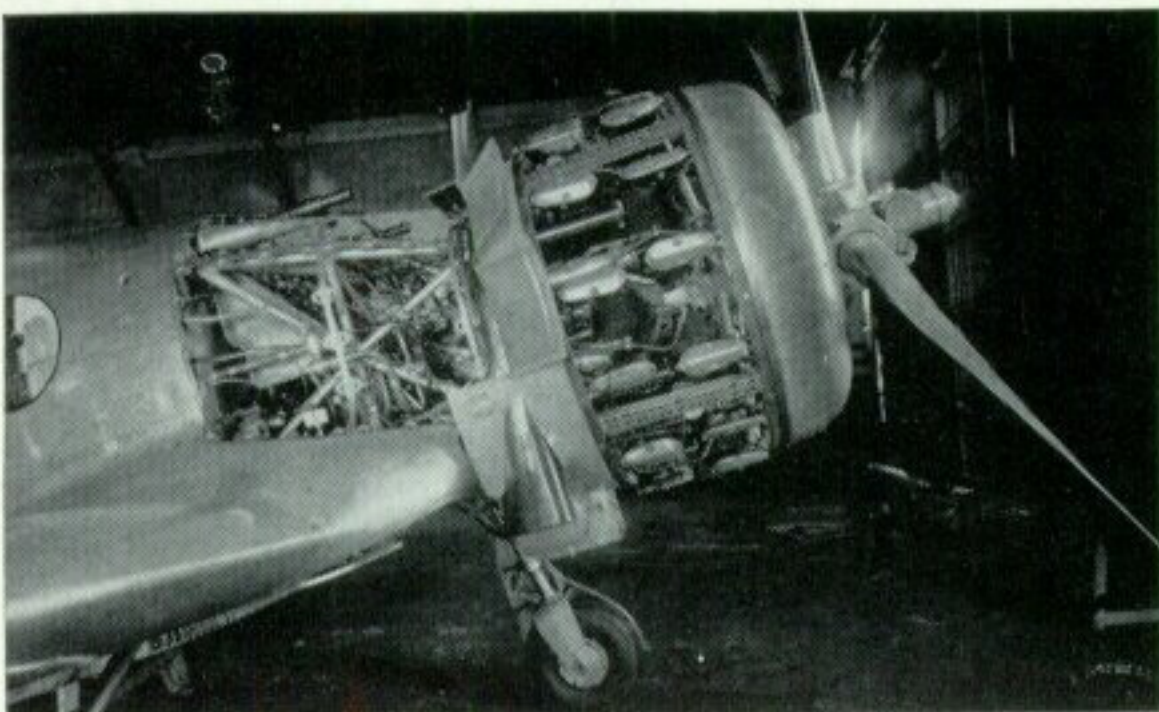
Left: Engine installation of the C.200. The characteristic "blisters" on the cowling panel were necessary to accommodate the rocker-boxes of the fourteen-cylinder Fiat A.74 R.C.38 radial powerplant. Right: Experimental semi-open cockpit canopy installed on one C.200, with rear-hinging top section. The reflector sight can also be seen in this photograph.
