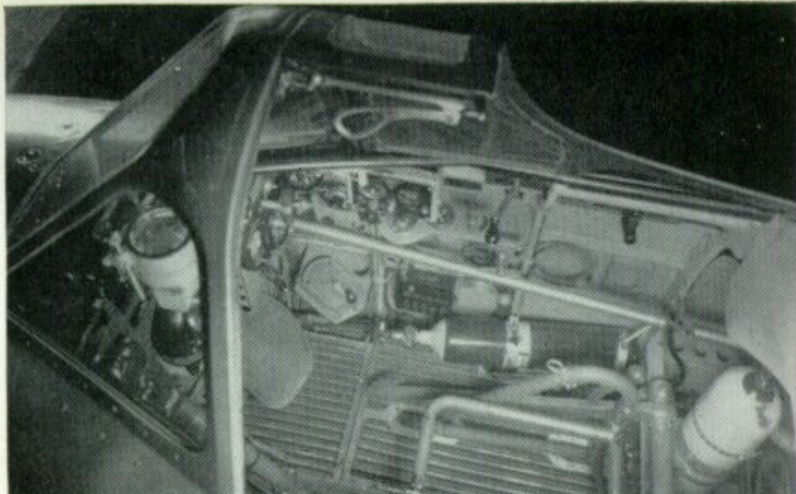
Left: A Saetta being run-up "on the bench" during systems tests; note the propeller spinner and the structure of the semi-retracted undercarriage. Right: The cockpit of a Macchi C.200 of the sixth production batch, seen here without the pilot's seat. Oxygen system and fire extinguisher are clearly visible.
